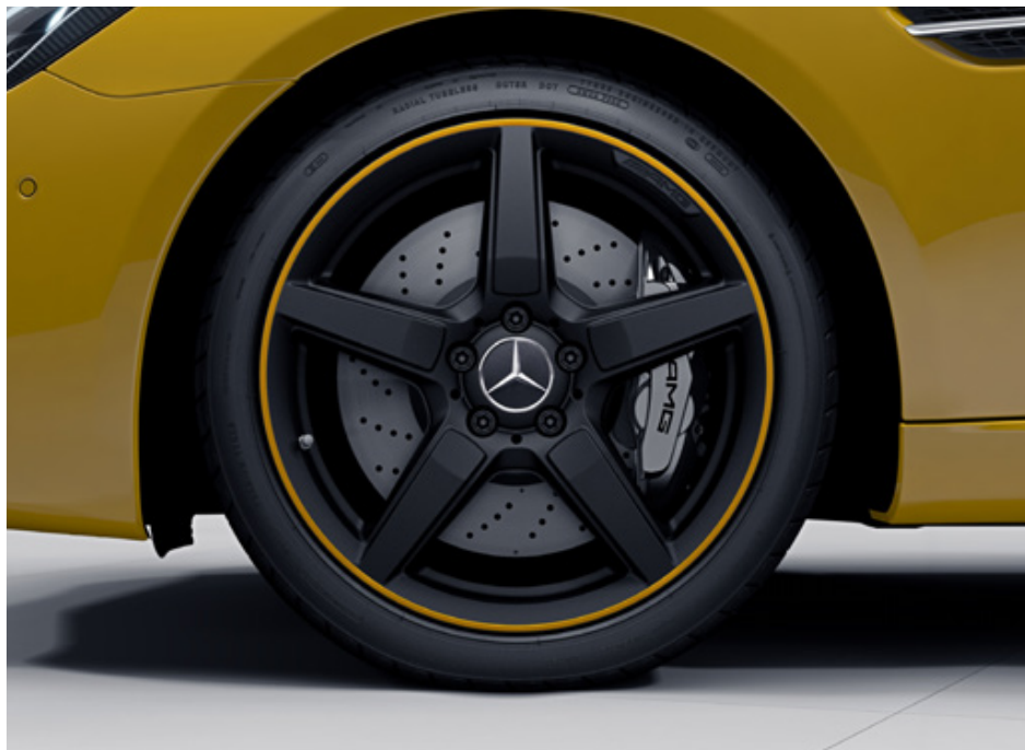
RGK 18" AMG bi-colour alloy wheels (4) – 5-spoke design painted matt black with yellow rim flange front: 235/40 tyres; rear: 255/35 tyres
