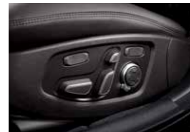
22-way automatically adjustable driver's seat (Modern ERGO Seat)
