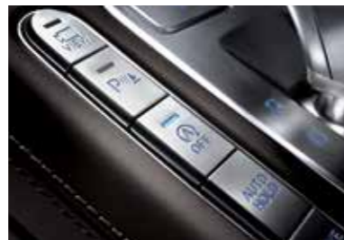
ISG system (idle control)
