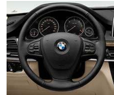
■ Leather steering wheel with multifunction buttons for operating the Cruise Control and the radio or telephone.
