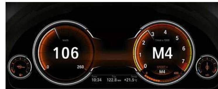
□ The Multifunctional Instrument Display 2 with Black Panel technology and a screen diagonal of 10.25" provides an impressive visualisation of the driving experience. Three different modes and their specific characteristics – each of which have their own colour scheme and graphic style – can be shown in the display: COMFORT, ECO PRO and SPORT modes.
