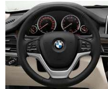
□ Sport leather steering wheel , black, three-spoke, with multifunction buttons and chrome inlay. ■ Servotronic adapts the steering power to suit the speed.
