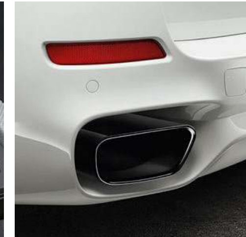
Exhaust tailpipe. The trapezoidal tailpipes on the left and right are encased in a black chrome trim.
