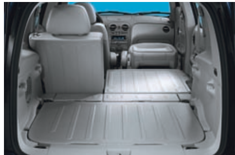
Composite seatbacks fold down to accommodate larger items and provide a durable surface when carrying cargo.
