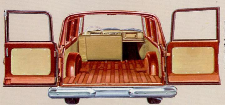
Loading the all new 'Jeep' Panel Delivery is no chore at all. Its big double rear doors swing all the way open to a high and wide 39½ in. by 55 in., the full inside height and width of the vehicle. Bed height is a short 23½ in. from the ground. There's a full 107 cu. ft. of usable cargo space—room to accommodate bulky loads of up to 1200 lbs. Yet unlike many competitors, when fully loaded, the 'Jeep' Panel Delivery still handles with ease, rides with unbelievable smoothness.
