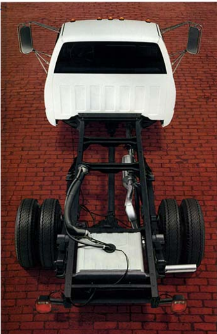
New Series 3500 HD 4x2 Chassis-Cabs with GVWRs up to 15,000 lb offer the highest load capacity currently available in the light-duty field.
