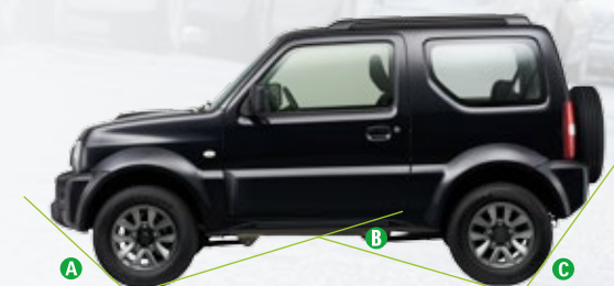
A 34° approach angle B 31° ramp breakover angle C 46° departure angle (default setting, unloaded Jimny)
