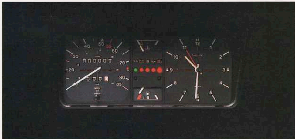
New instrument panel has light-emitting diodes replacing ordinary lamps. Be sure to see it.
