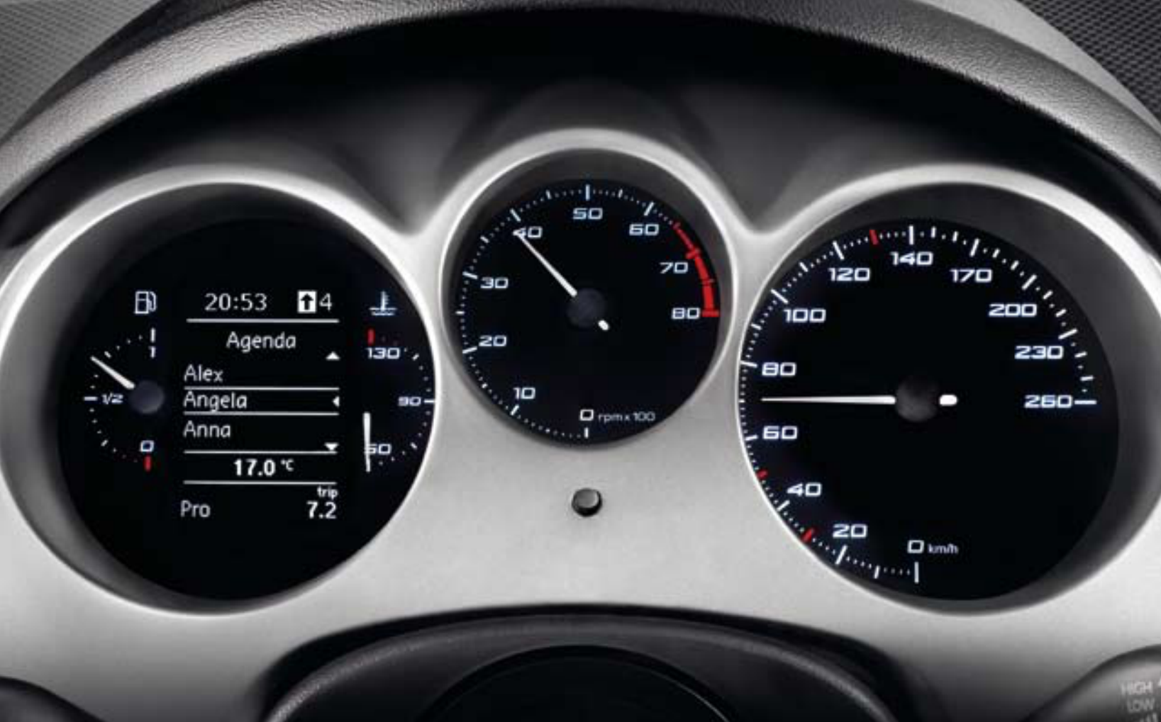
New instrument cluster with white graphics. A gear-shift indicator* ensures either a more sporty drive or maximum efficiency.
