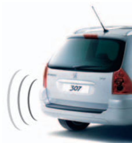
Parking Aid To help you manoeuvre more safely; the system emits audible beeps when the car approaches an obstacle. The parking aid can be fitted without the need to drill the rear bumper. (Please note the system will not function whilst towing).
