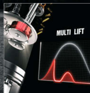
MULTI LIFT Multiple valve opening during the same cycle Minimum torque and power E.g. city driving
