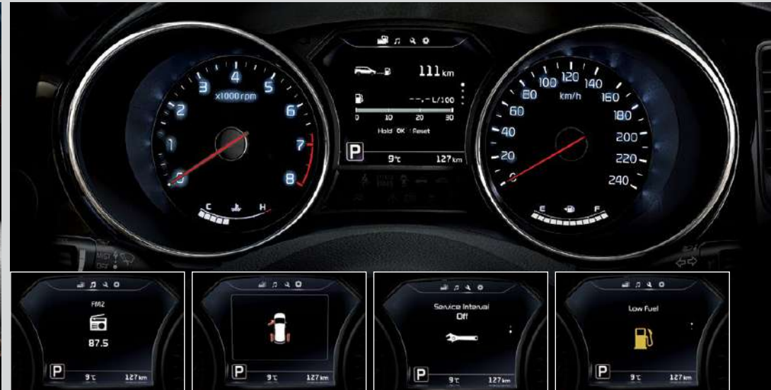
Supervision cluster (7" colour TFT LCD) A high-visibility display located in the centre gauge cluster provides useful, on-demand trip computer information graphics such as distance to empty, average and instant fuel consumption and outside temperature.
