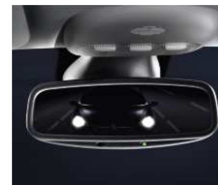
To avoid any risk of being dazzled an electrochromic rear view mirror ◊ becomes tinted if the light level decreases.
