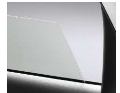
The laminated acoustic side windows o give excellent sound insulation along with added safety.
