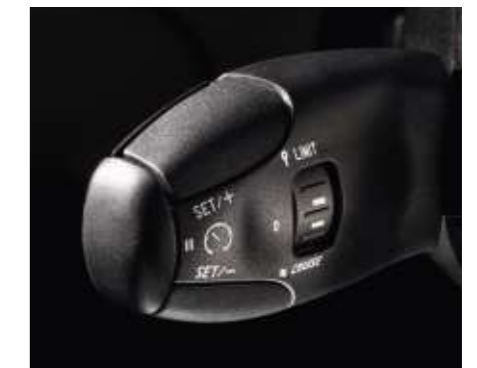
A speed limiter coupled with the cruise control o prevents you from going beyond your set speed unless you deliberately "kick-down" the throttle.
