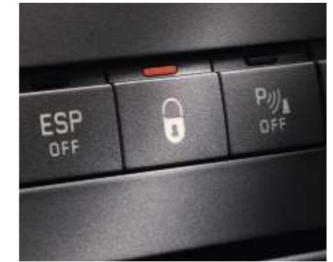
Above 6 mph the doors are locked automatically.
