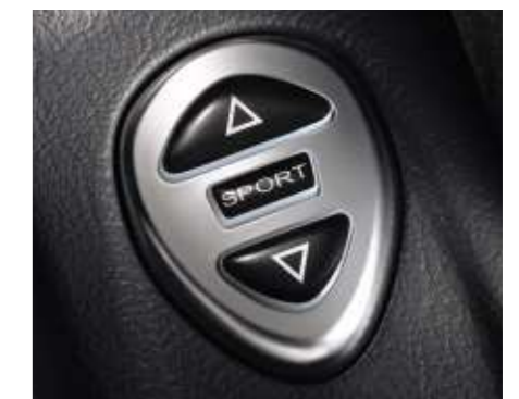
With a touch of a button, Hydractive 3 can be switched to a 'Sport' setting o to promote the suspension's more dynamic driving characteristics.
