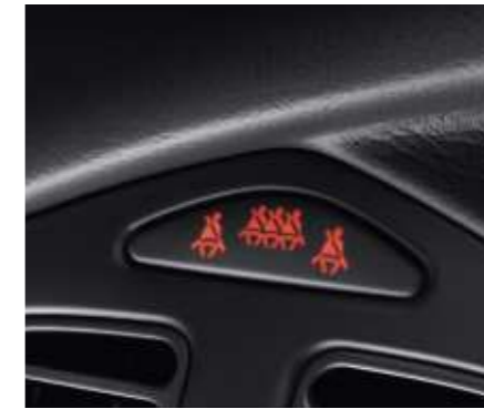
For better safety a warning light flags up any non-fastened seat belts
