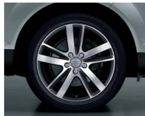
Cast aluminium wheels, 10-spoke V design, anthracite, partially polished, size 9 J x 20 with 275/45 R 20 tyres
