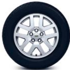
18 inch 5-spoke Alloy Wheels Tyre Specification: 255/60 AT/H Rated
