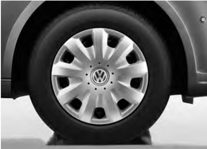
STEEL WHEEL WITH STYLISED WHEEL COVERS – 6J x 15" (195/65 R15) – STANDARD ON THE TRENDLINE
