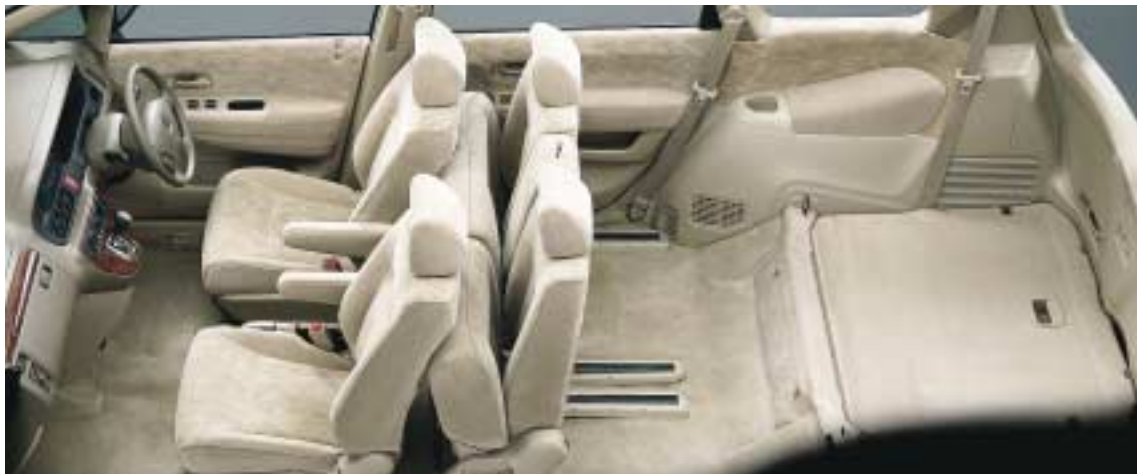
The third row 'sofa' retracts into the floor for flat cargo space. The spare tyre is underneath.
