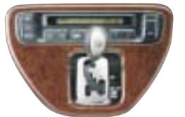
The race-bred S-Matic gear lever is mounted on the instrument console panel rather than the floor or steering column for superior driver comfort and control.
