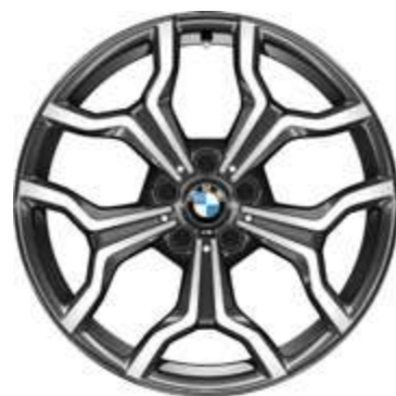
2QL 19" M LIGHT ALLOY WHEELS Y-SPOKE STYLE 722 M 8J x 19 / tyres 225/45 R 19
