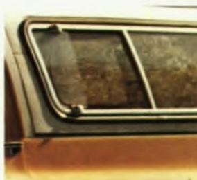
Sliding side windows in removable plastic top.
