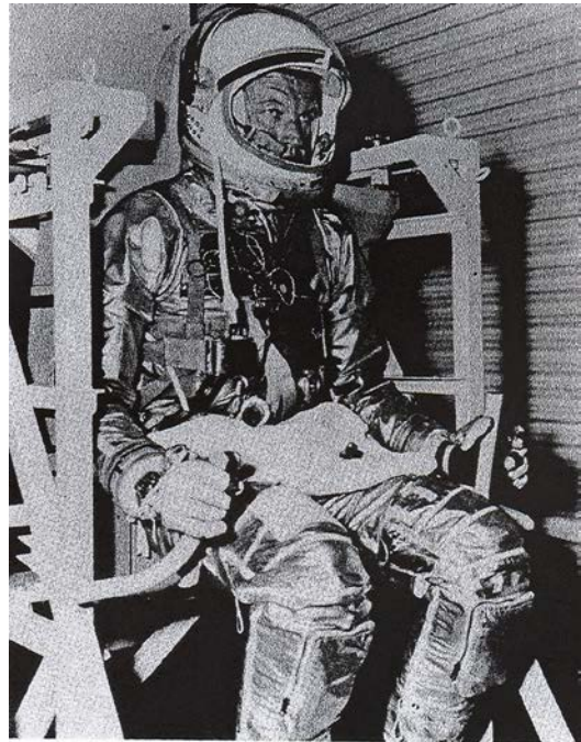
Fig. 139. Astronaut L. Gordon Cooper, Jr., in contour couch during weight and balance tests. Hangar "S" - White Room - Cape Canaveral, Florida.
