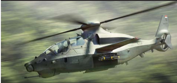
Bell 360 Invictus Tandem cockpit, articulated main rotor, wing, canted ducted tail rotor and supplemental power unit.
