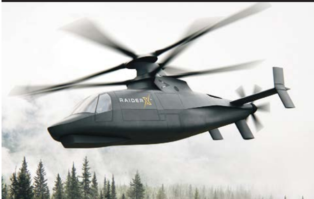
Sikorsky Raider X Side-by-side cockpit, coaxial rigid rotors and pusher propulsor.
