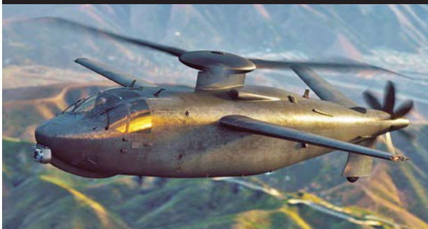
Karem Aircraft/Northrop Grumman/Raytheon AR40 Side-by-side cockpit, active rigid rotor, tilting wing and swiveling tail-rotor/propulsor.
