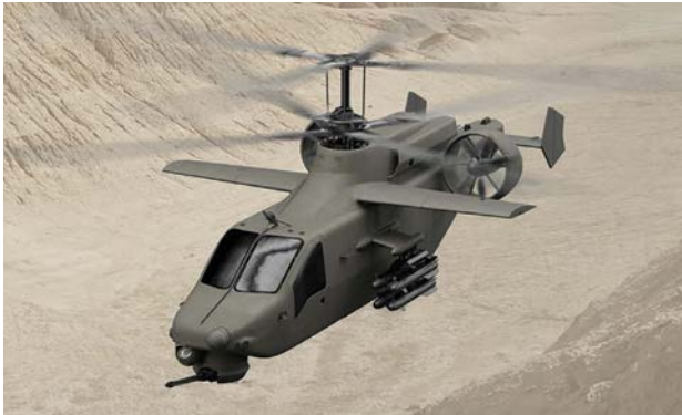
AVX Aircraft/L3Harris Technologies Compound Coaxial Helicopter (CCH) Side-by-side cockpit, articulated coaxial rotors, wing and ducted fans.
