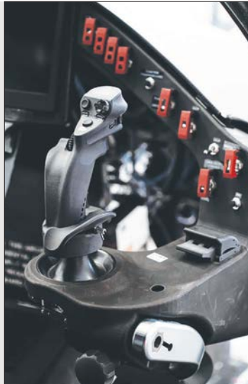
The right-hand inceptor controls ascent and descent.
