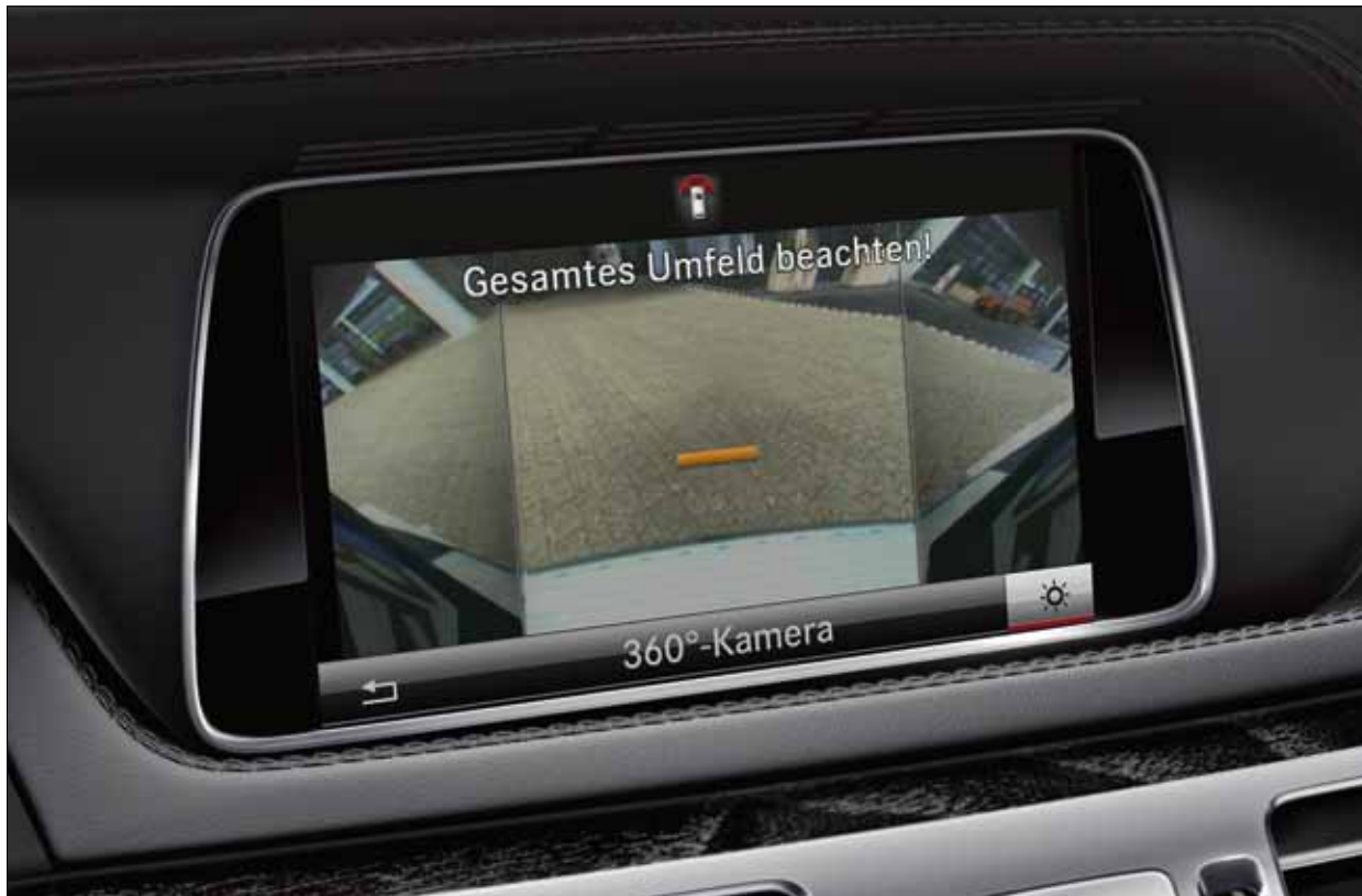
The 360° camera system uses four cameras to provide views all around the vehicle.
