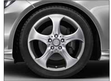
5-spoke light-alloy wheels with 245/40 R 18 front tyres and 265/35 R 18 rear tyres (option, Code R08/52R).
