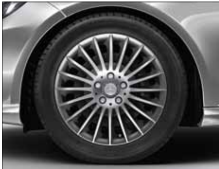
Multi-spoke light-alloy wheels with 245/45 R 17 tyres (standard on ELEGANCE for 4- and 6-cylinder versions and for all 4MATIC models except E 500 4MATIC, Code 08R/04R 1 ).
