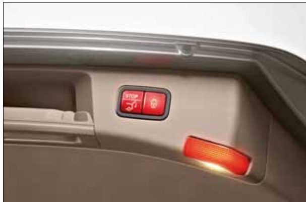
The EASY-PACK tailgate can also be opened and closed in a lower position at the push of a button.
