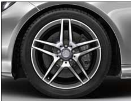
5-twin-spoke AMG light-alloy wheels with 245/40 R 18 front tyres and 265/35 R 18 rear tyres, 4MATIC with 245/40 R 18 tyres all round (part of AMG Sports package, Code 660/794).
