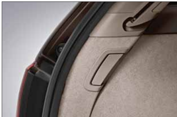
Release handle makes light work of folding down the rear seat backrests.
