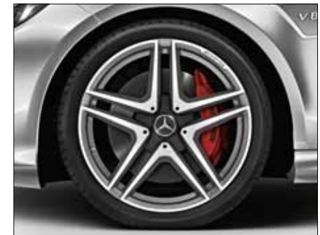
5-twin-spoke AMG forged wheels with 255/35 R 19 front tyres and 285/30 R 19 rear tyres, painted titanium grey with high-sheen finish (option for AMG models, Code 785).
