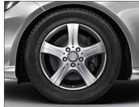
5-spoke light-alloy wheels with 245/45 R 17 tyres (option for 4- and 6-cylinder models, Code 02R).
