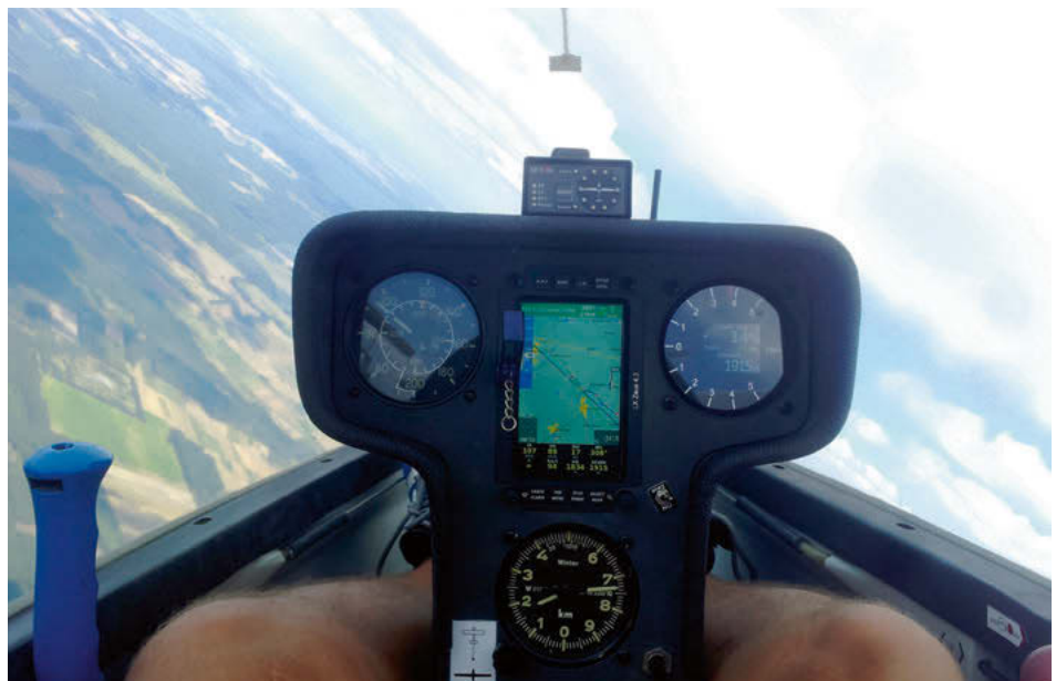
The 4.3 inch version of the LX Zeus installed in DG-101G during the Junior Worlds (Toni Šibanc)
