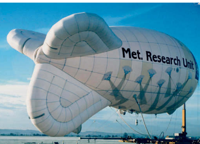
Figure 4: A kite balloon tethered by wire rope and flown at a height around cloudbase is in great danger of being struck by lightning
