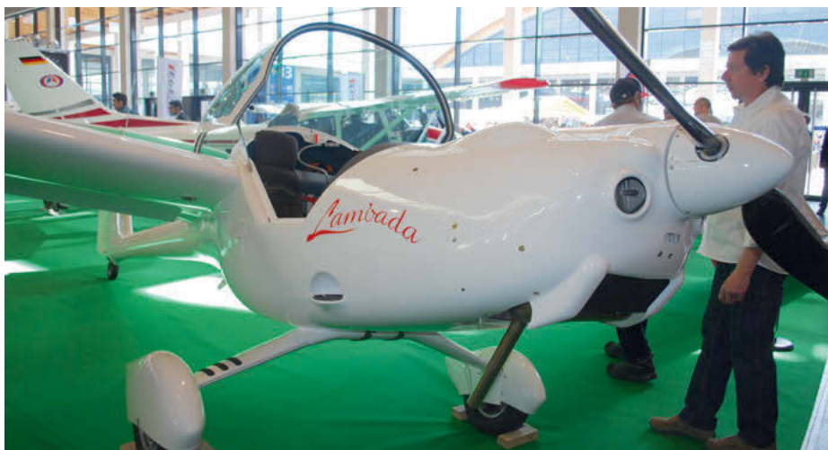
The LAMBADA S-LSA motorglider, not certified in the UK, has the option of 13m or 15m wingspan. It can be fitted with a towhook and aerotow tests have been successfully conducted in several countries, with various glider types up to 650 kg MTOW. www.adcompair.com
