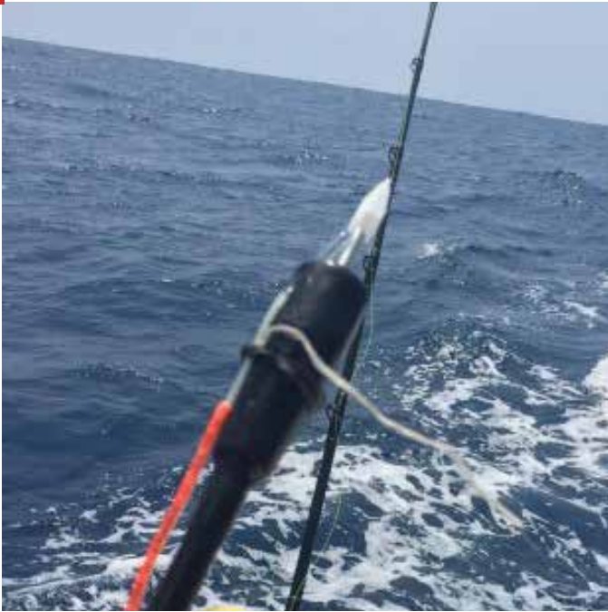
Piece of dental floss attached to a rubber band makes gripping easier when applying tag to tagstick.
