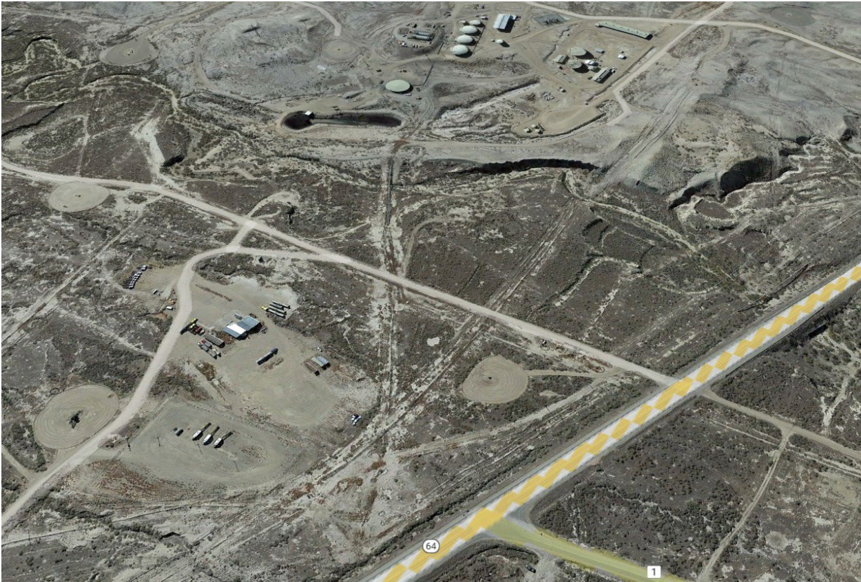
Typical part of the Rangely oil and gas field. Circular bare patches are places where wells have been drilled. Google Earth image.
