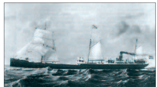
1886 Gluckauf this ship is considered the first modern tanker: oil carried right out to shell; cofferdams at each end of cargo section; cargo pumps for loading/discharging
