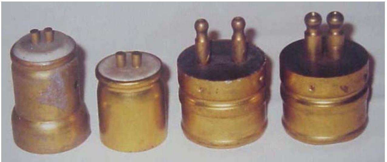
From left, two Westinghouse Stopper bases, Mogul Heisler round pin base, Mogul Bernstein round pin base
