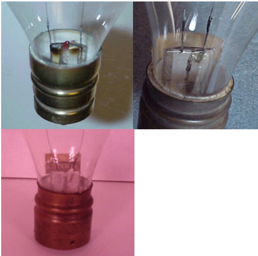
The porcelain-insulated Westinghouse-based lamp shown to the left has no label; the red fibre-insulated Thomson-Houston- based lamp in the center has a label stating
