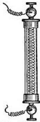
FIG. 138.—De la Rue's Enclosed Incandescing Metallic Wire. Note the fact that this form of incandescing metallic wire gave more light both because of its spiral form and from the fact of its being enclosed.
