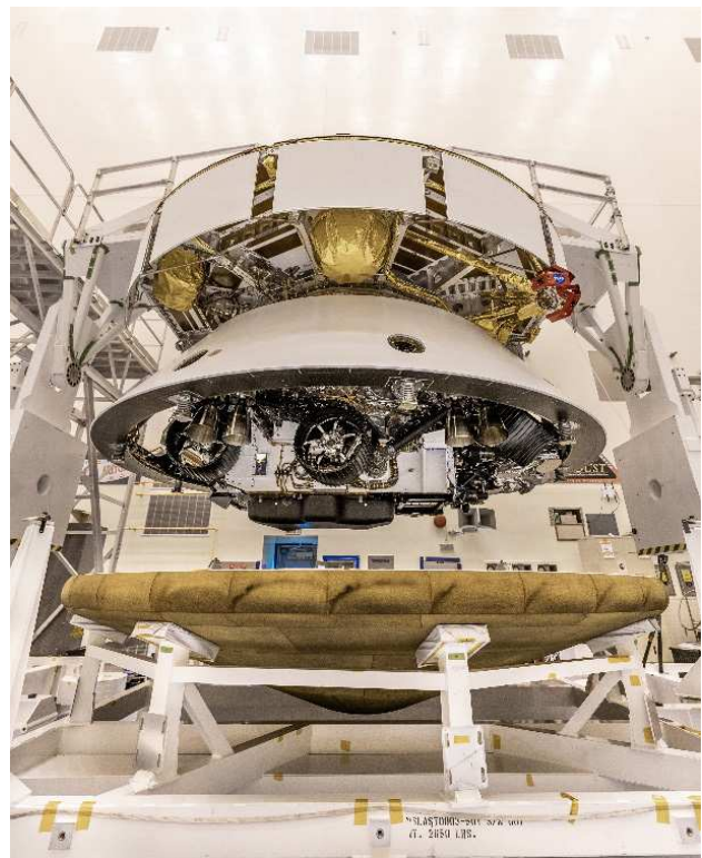
(Left) Perseverance rover, with all MEDA sensors, during heat shield installation, (Right) Mars 2020 mission with the Perseverance rover lifts off, July 30, 2020
