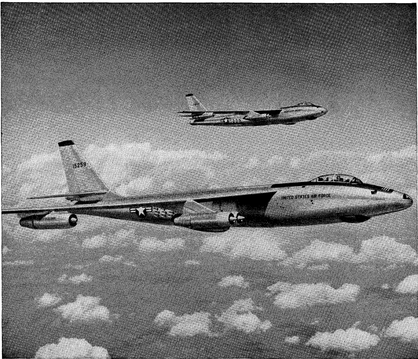
Foreground: Boeing RB-47E, world's fastest day-or-night long-range reconnaissance plane. Background: Standard B-47E six-jet bomber.
