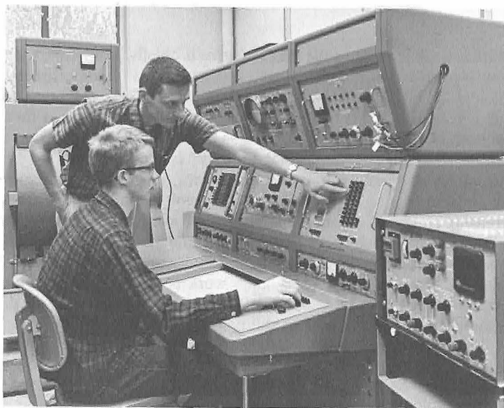
Undergraduate research student operating a digital frequency sweep nuclear magnetic resonance spectrometer
