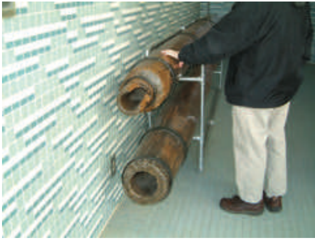
Figure 5 - Cedar logs and pump patented by Benjamin Franklin.
