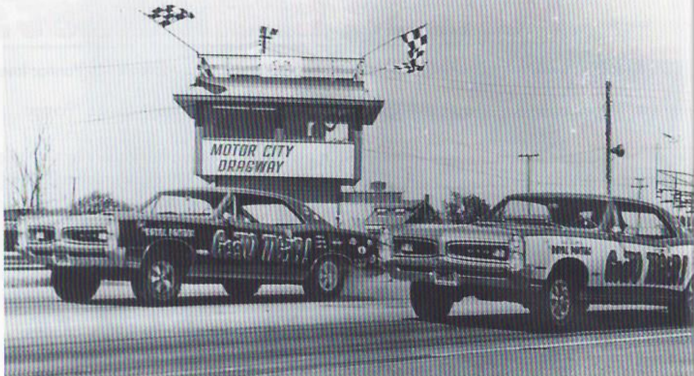
Both of the Tigers were equipped with blueprinted 421 HO Tri-power engines, M21 four-speed manual transmissions, 3.90:1 Safe-T-Trak rears and M&H slicks.
