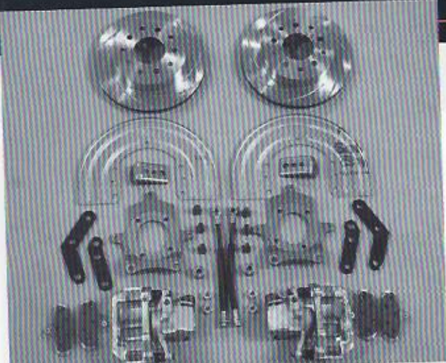
Rear Disc Brake Conversion Kit No. A 125-3 for '62-'74 GM 10- and 12-bolt rearends is the customary upgrade for Pontiac. The kit includes rotors, calipers with built-in parking brakes, dust shields, brake lines, adapters, mounting brackets, bolts and hardware, and detailed step-by-step instructions. Since the Moser 12-bolt rearend on the GeeTO Tiger was assembled with big Ford bearings and housing ends, we opted for the rear conversion No. A 110-2 kit with GM pattern rotors.
