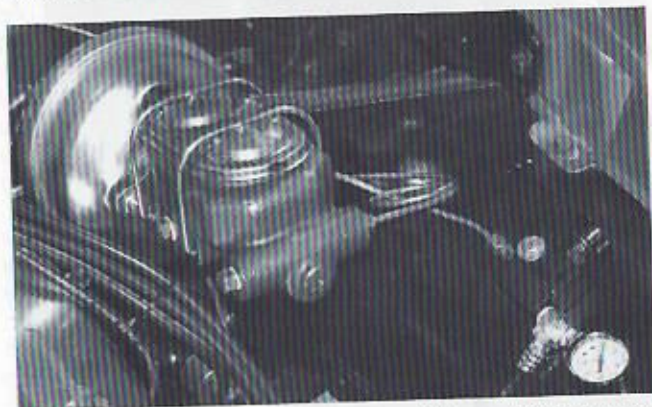
The disc-brake kit comes with a master cylinder and 9-inch power booster. To clear the tall valve cover, a 7-inch booster was used. The adjustable proportioning valve with gauge is then installed in the rear brake line. Note the vacuum hose extending from the forward-mounted vacuum pump.
