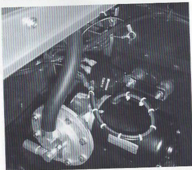
Since the battery had been relocated to the trunk, the vacuum pump was mounted with the supplied insulators to the core support. The vacuum line was routed atop the fender well rearward to the booster.
