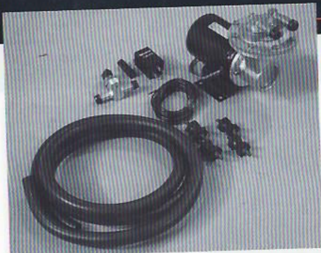
The Vacuum Pump Kit No. 28146 includes the vacuum pump, relay switch, distributor vacuum switch, wiring, rubber insulators and a length of vacuum hose.
