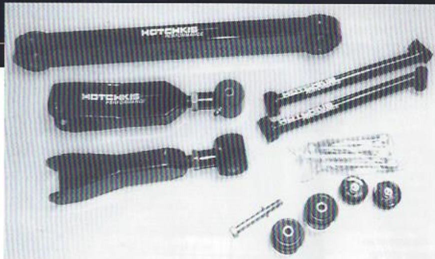
Hotchkis Engineering supplied the '64-'67 GM A-body rear-suspension components, including lower bar (top), adjustable upper bars (left), upper and lower cross-braces (right) and bushings (lower right). Not shown is the rear sway bar.
