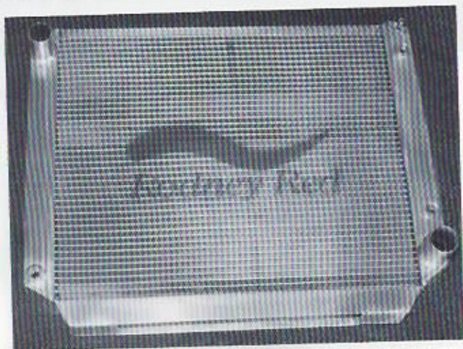
Shown is the custom-fabricated Rodney Red aluminum radiator. Specifically designed for the '66-'67 GTO chassis, this efficient heat exchanger saves quite a few pounds over a standard four-core factory version.
