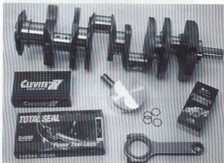
Here's the JBP Tiger engine's rotating assembly with new JBP crankshaft, Eagle rods, JBP/Ross pistons and premium bearing kit. There's 15 percent more steel in the crank's composition, exceeding factory specs.
