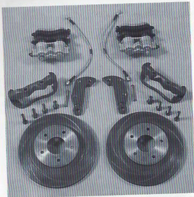
Stainless Steel Brakes' Super Duty Front Disc Conversion Kit No. A 123-6 features twin-piston aluminum calipers, 12-inch vented and slotted rotors, mounting brackets, pads and hardware. The kit also includes an adjustable proportioning valve, adapter lines, stainless steel flex hoses, master cylinder, 9-inch booster, seals, bearings and easy-to-read instructions.
