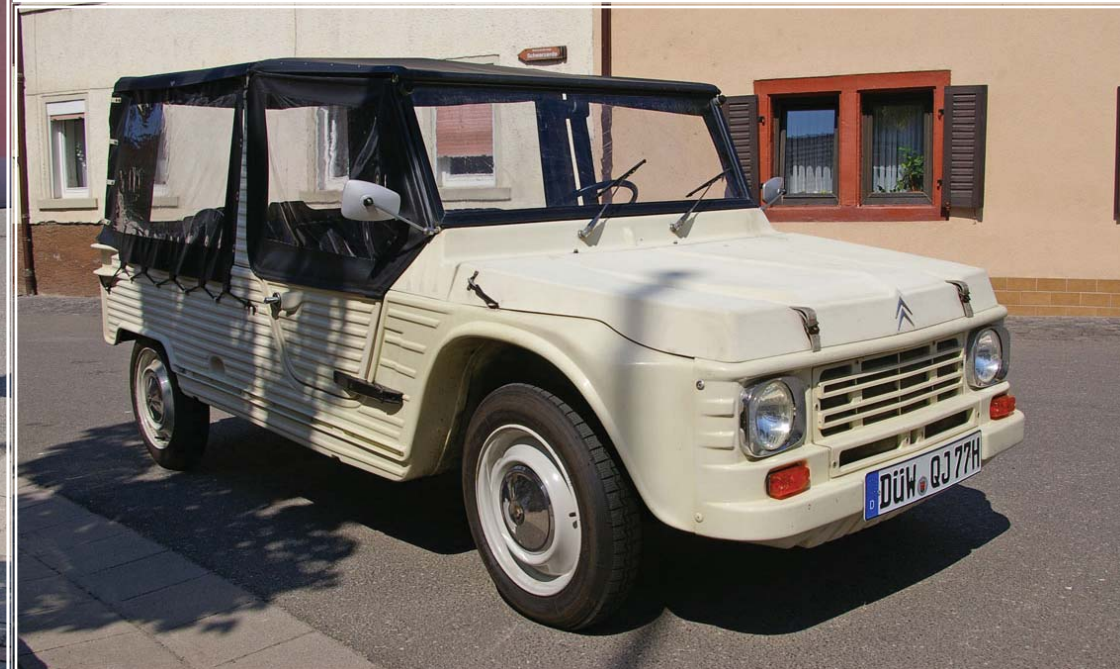
The Citroën Méhari has a tubular frame as well as a steel floorpan to support all the mechanical components as well as the novel plastic body
