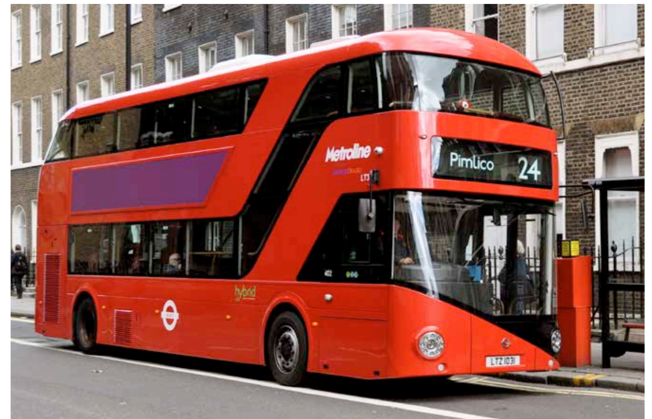
London's new Routemaster hybrid double deck bus with three doorways and two staircases accommodates 80 passengers; September 16, 2013, at bus stop in Bloomsbury, London, UK. © Ron Ellis / Shutterstock.com
