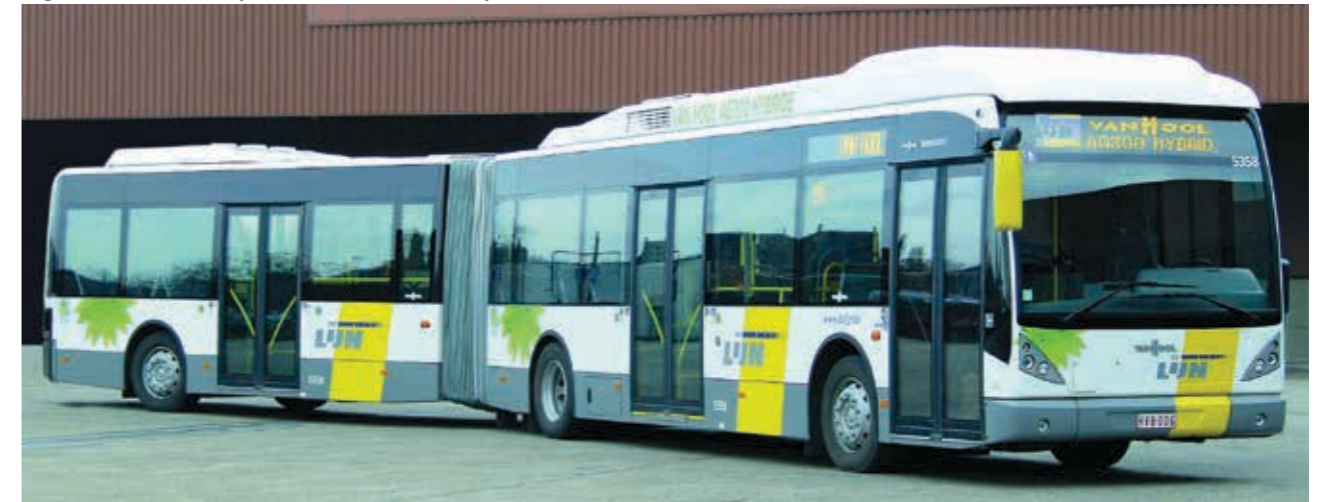
Figure 13. Serial hybrid diesel/electricity bus
