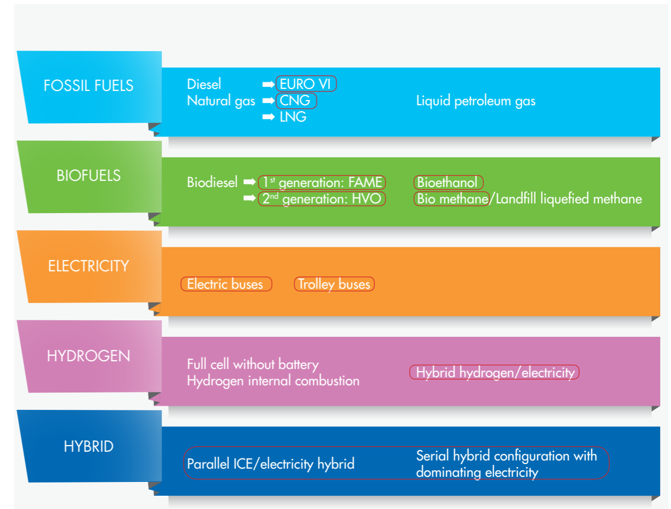
Figure 4. Possible and most promising bus technologies for different energy carriers
