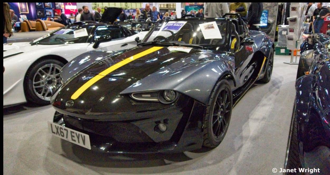
Zenos E10 R - 2.3 litre turbocharged EcoBoost engine and 6 speed manual gearbox. 0-60 mph in 3 seconds
