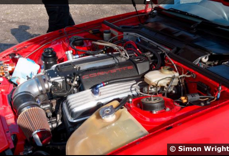
Porsche 944 Turbo notfitted with 5.7 litre Chevrolet Corvette engine
