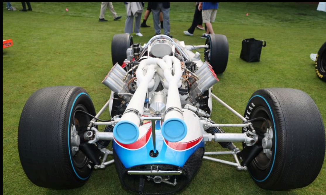
AJ Foyt's 1964 Sheraton Thompson Special with oval circuit suspension offset, really a Lotus 34
