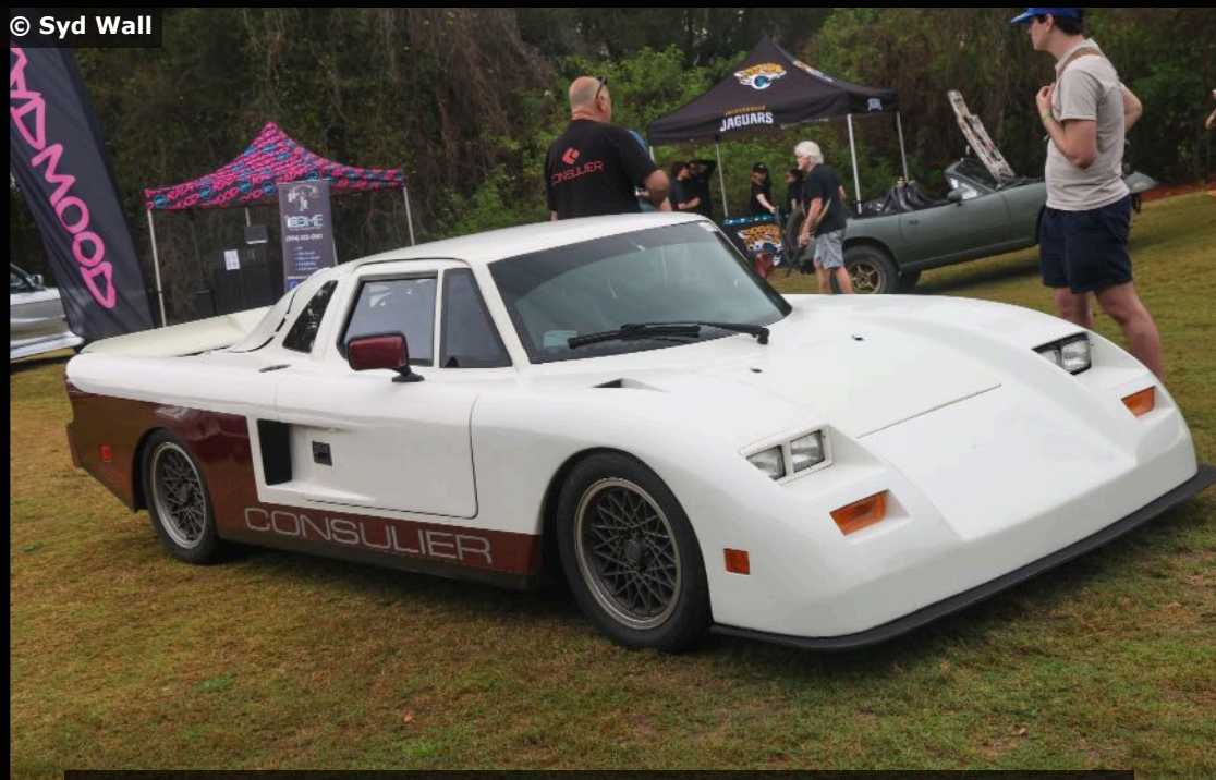
The Consulier GTP, the first carbon & Kevlar-bodied production vehicle with no structural metal - the company morphed into the more widely known Mosler.
