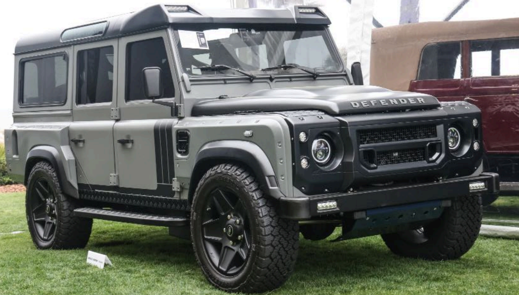
A 1987 Land Rover Defender 110 sold for $196,000? 6.2 litre Chevrolet LS3 engine, 6 Speed auto box and adjustable air suspension
