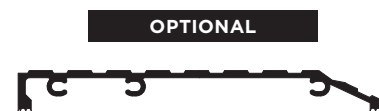
1/2" Tileback Aluminum Saddle Threshold (ADA) Tileback sill only available in 5" width. For use on a 4-9/16" jamb only.
