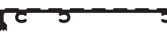
1/2" Tileback Aluminum Saddle Threshold (ADA) Available in 4-1/4" and 6-1/4" widths. Inswing use only.
