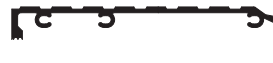
1/2" Tileback Aluminum Saddle Threshold (ADA) Available in 4-1/4" and 6-1/4" widths. Inswing use only.
