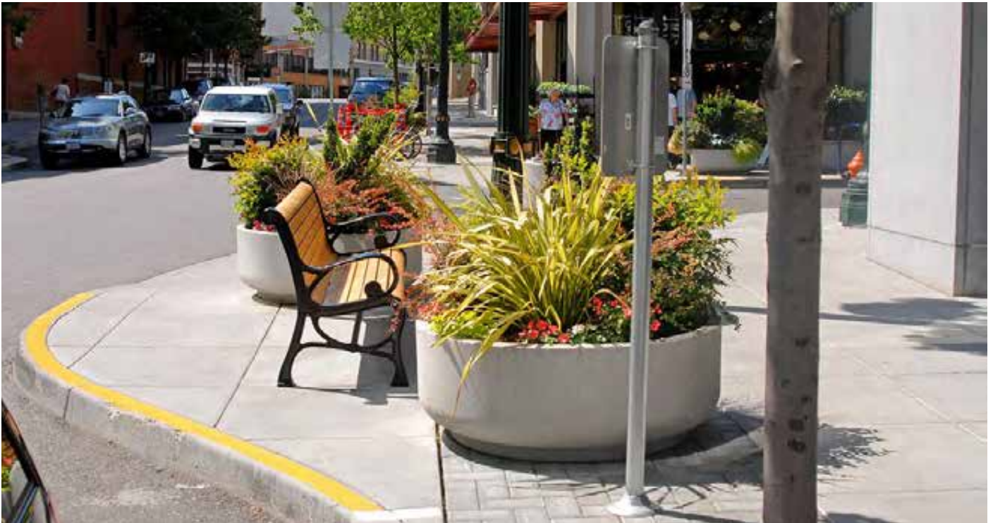
Bulb-outs at street corners can provide pedestrian amenities, such as seating, lighting, and planters on otherwise narrow sidewalks.
