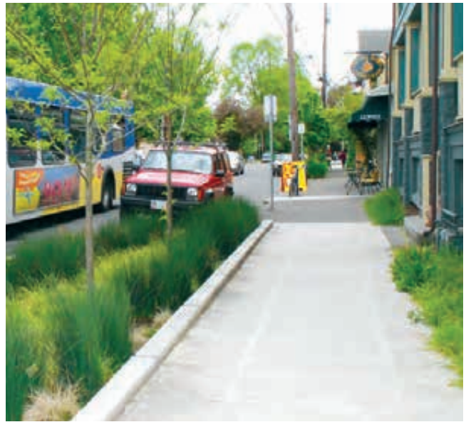
Street trees and rain gardens define the street edge for pedestrians while helping reduce the heat island effect, providing shade, and filtering stormwater runoff.
