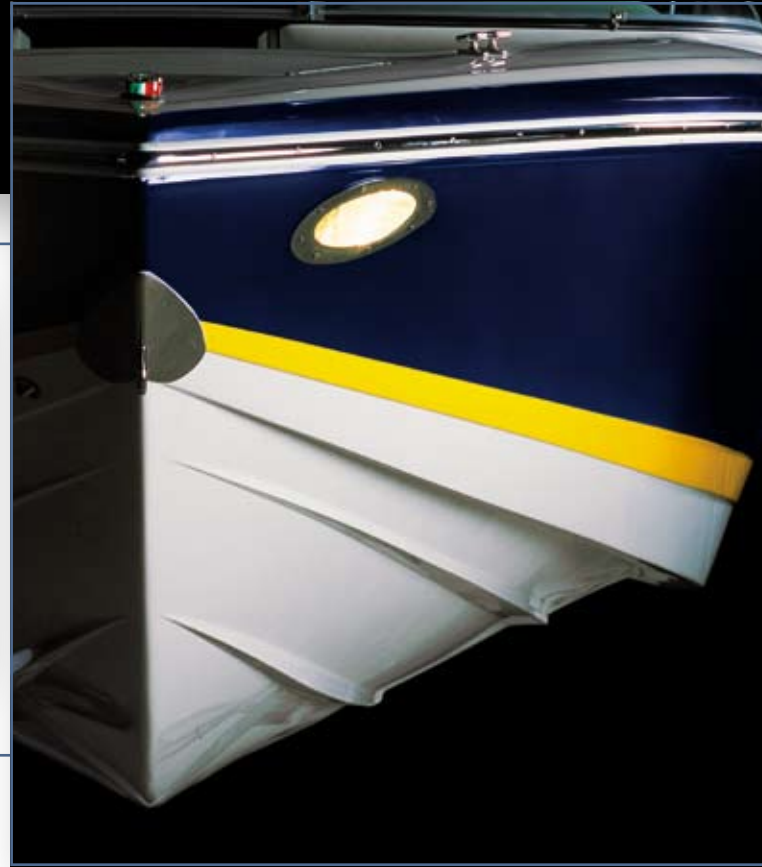
The deep-V shape and the reverse chines of the hull make the Cobalt ride smooth, solid and true with effortless total control.
