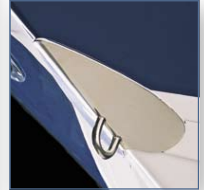
Another industry first was the added protection of a solid stainless steel bow scuff plate.
