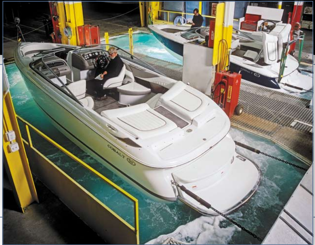
Every boat produced is put through a thirty point check while run under load for thirty minutes in the test tank.
