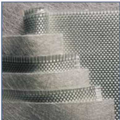
Multiple layers of hand laid fiberglass woven roving and mat give the ultimate strength fiberglass parts.
