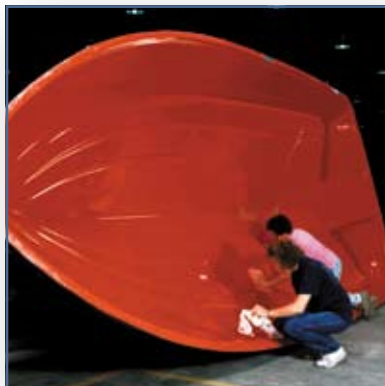
Hand waxing of the molds for a flawless no buffer-swirl finish in the final hull.
