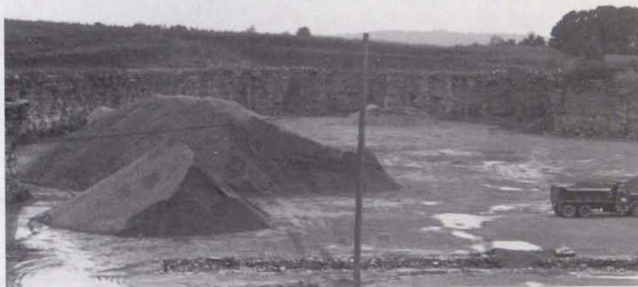
Figure 16. Spring Grove Underpass Quarry of the Roverud Construction Co. Until a few years ago, this locality was marked by a Milwaukee Railroad bridge over the highway and hence the name. Quarry shows all but 2'4" of the Platteville Limestone and most of the 23 feet of Decorah Shale present in this township. This thinning is due to the location on the crest of a small (50 feet in amplitude) anticline oriented N. 40° W.
