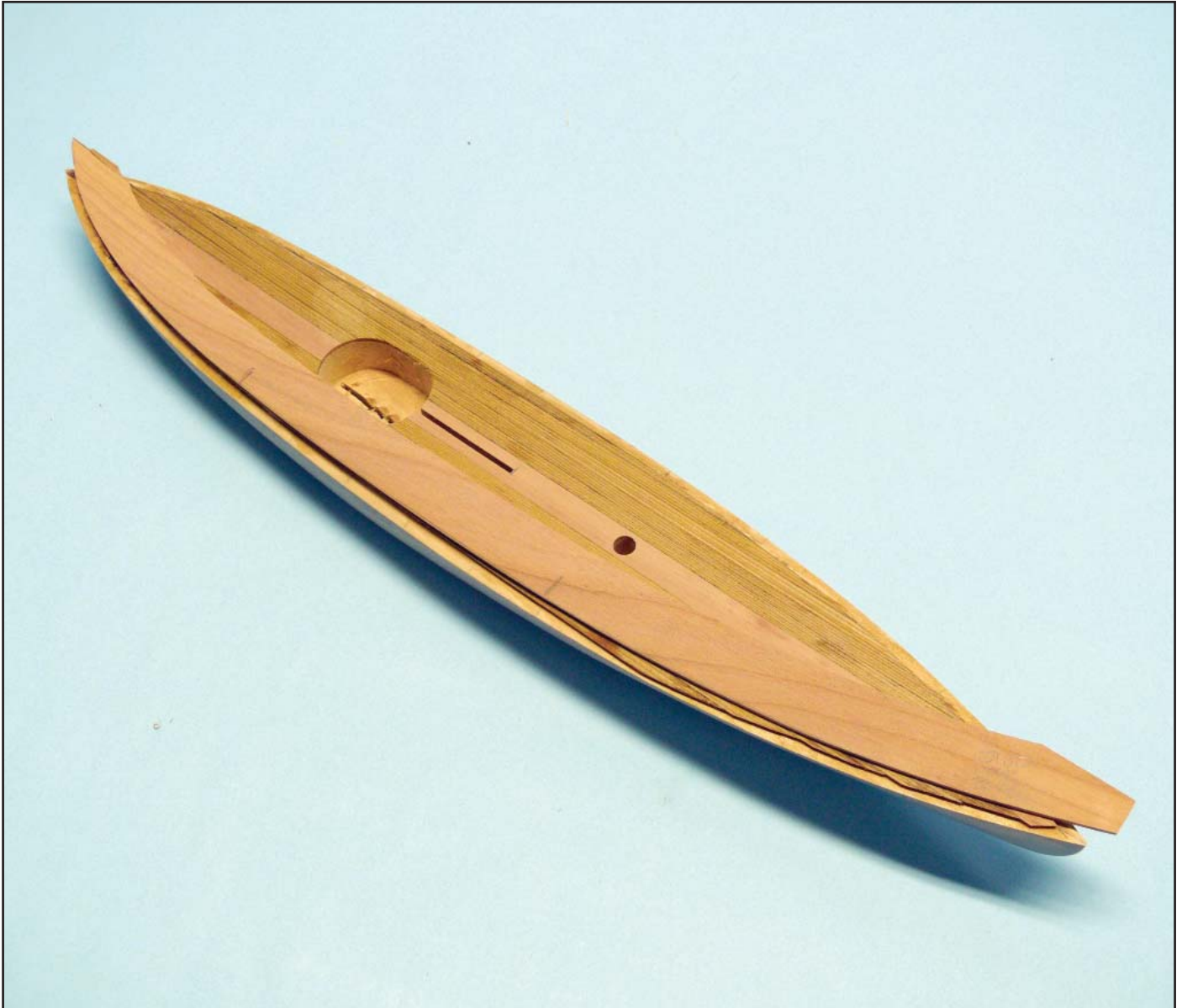
22. The template for cutting the deck planking.
