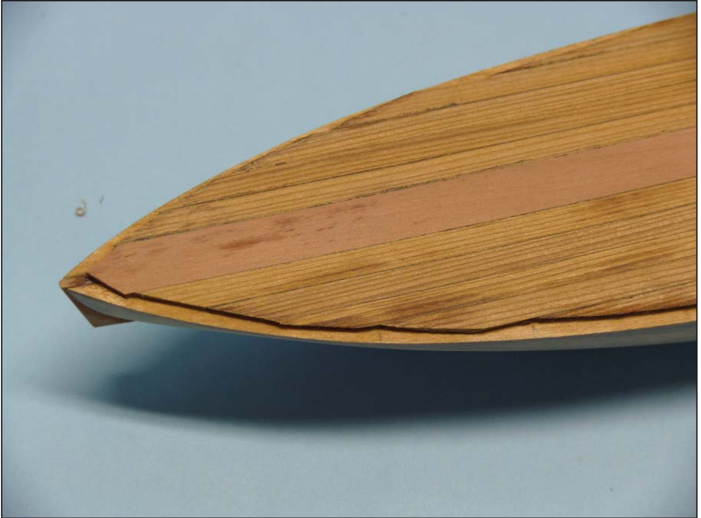
19. Decking. The pear king plank and cedar deck planks are glued in place.
