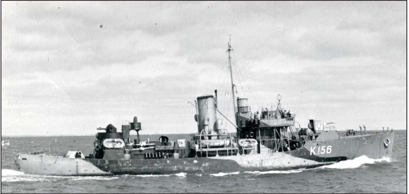
Figure 3 (April 1942): After refitting at Liverpool, Nova Scotia, Chicoutimi's foremast has been moved aft and the bridge expanded. There are 20-millimeter cannons on the bridge and a 2-pounder in the aft tub. A 20-inch searchlight has been mounted forward of the gun tub. There are now four depth charge throwers. The galley stack now rises up the funnel instead of the aft side of the bridge. The structure between the mast and bridge is the British Type 271 radar. The SW radar was retained but its older Yagi antenna has been replaced at the masthead by four dipoles configured in an 'X'. Gun shield art has been added: Bugs Bunny chewing on a U-boat superimposed on an Indian head, saying "What's Up Doc?". The camouflage is an RN pattern.
