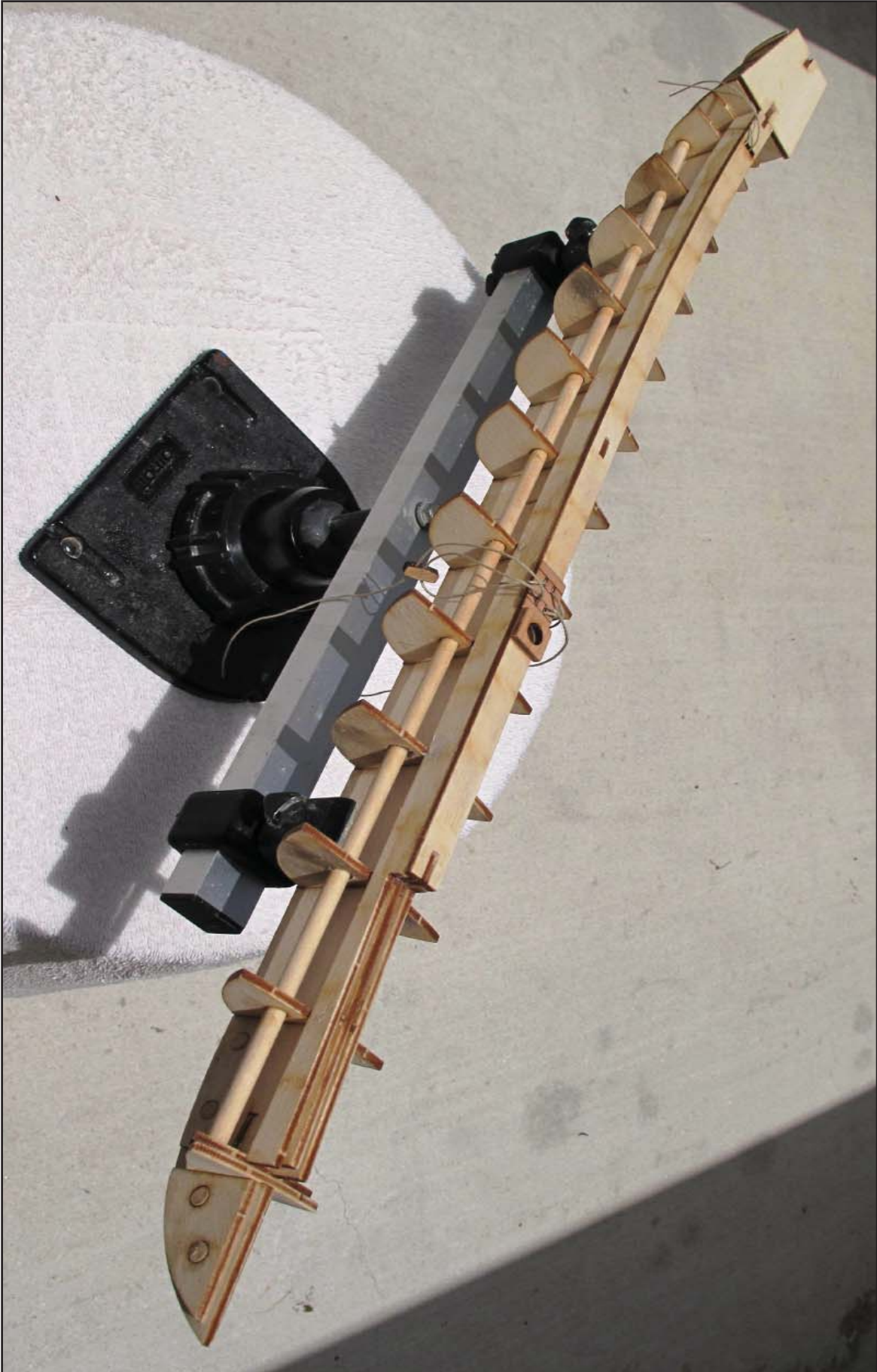
5. Completed keel assembly prior to the installation of the planking and decking.
