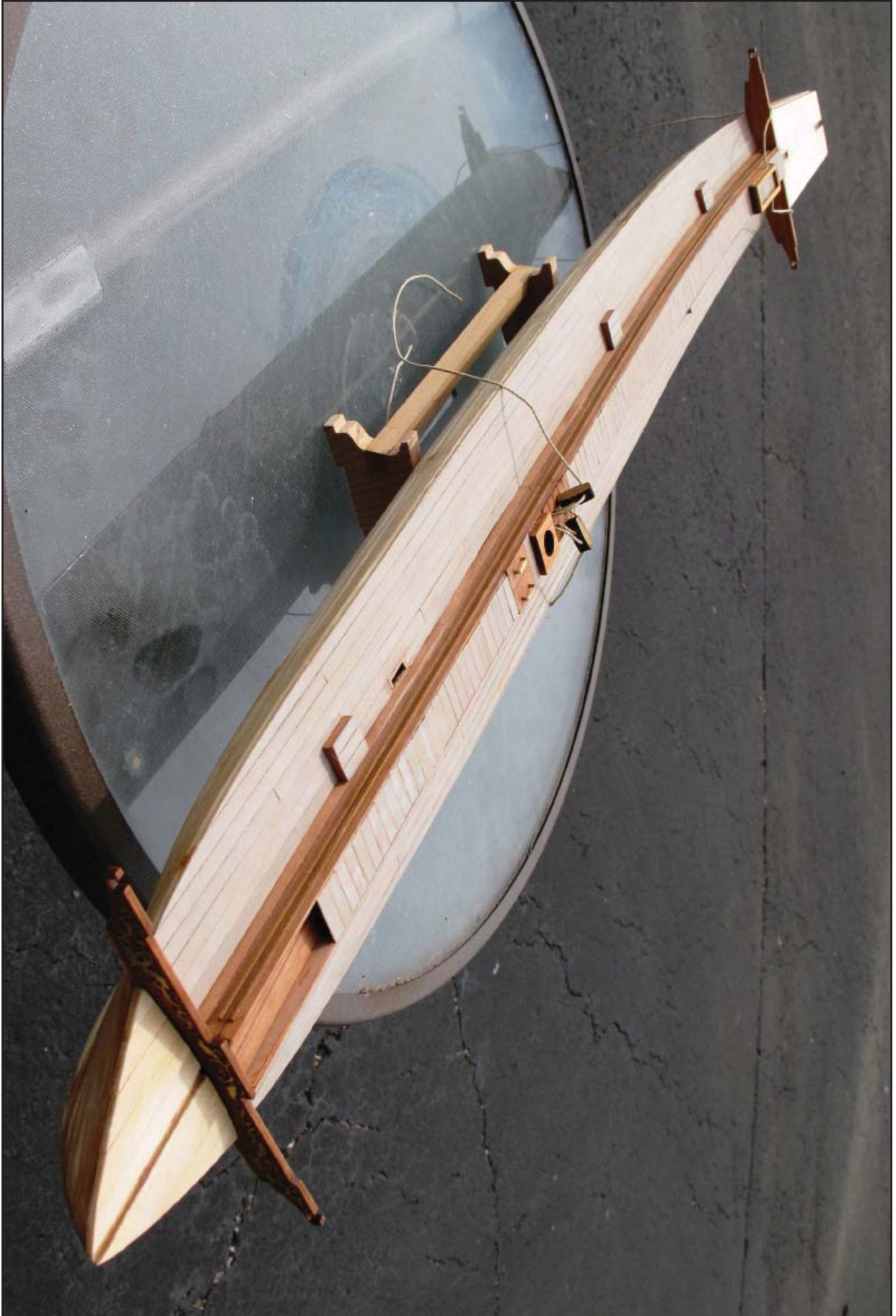
7. Hull showing the finished decking and the yokes that will support the rowing frame.
