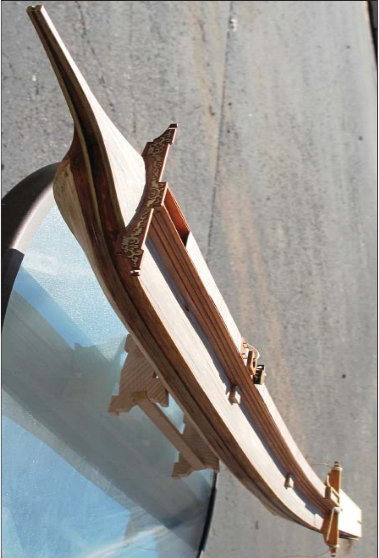
8. View of the model showing the spur, finished fore decking and hull planking.
