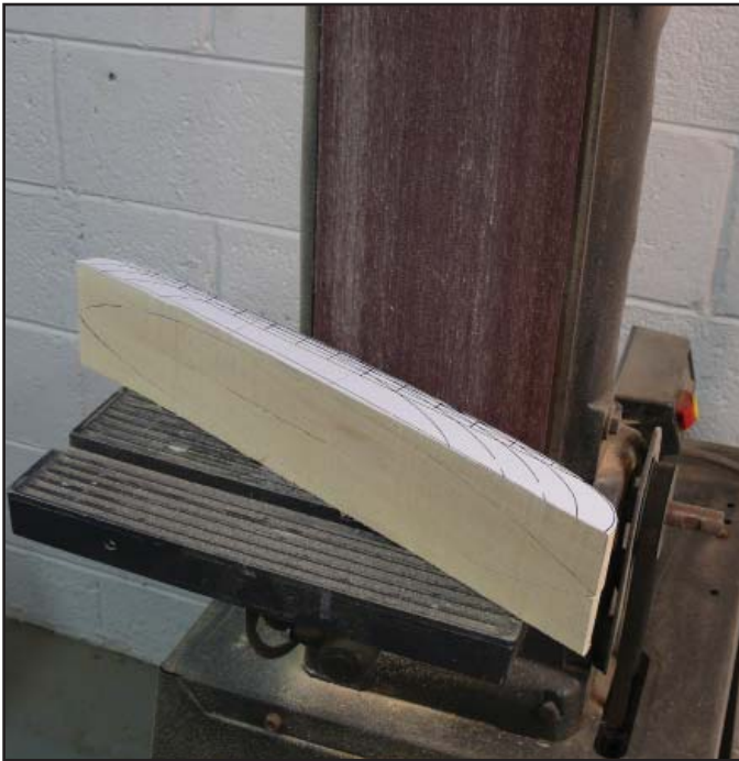
10. Sanding the bottom of the blank. The top and both sides of the profile have yet to be done.
