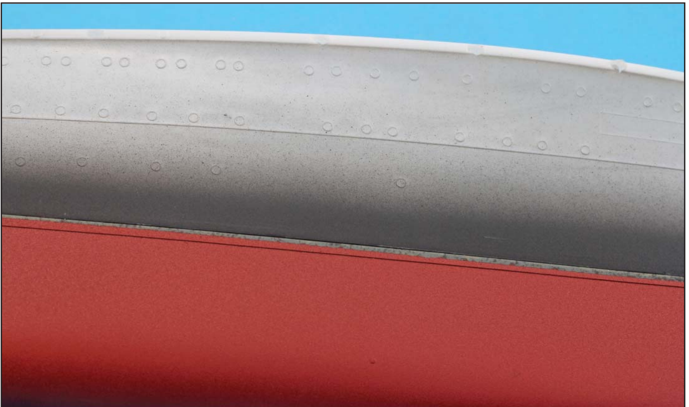
10. Mask removed from upper hull. Note the waterline tape showing the lower half with the lower hull color.
