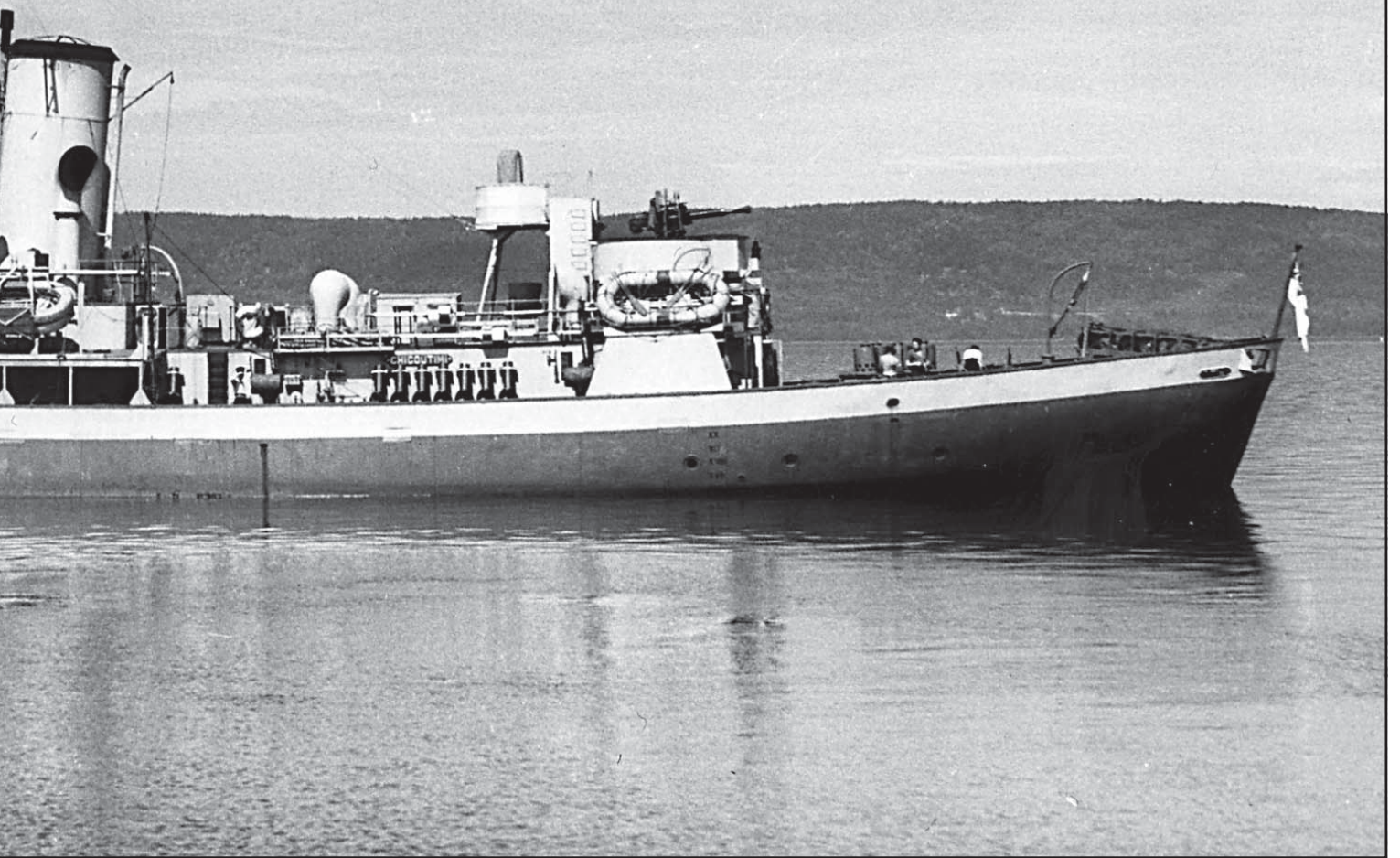
extra rafts port side and a 27-foot motor whaleboat to starboard, the new standard corvette arrangement.
