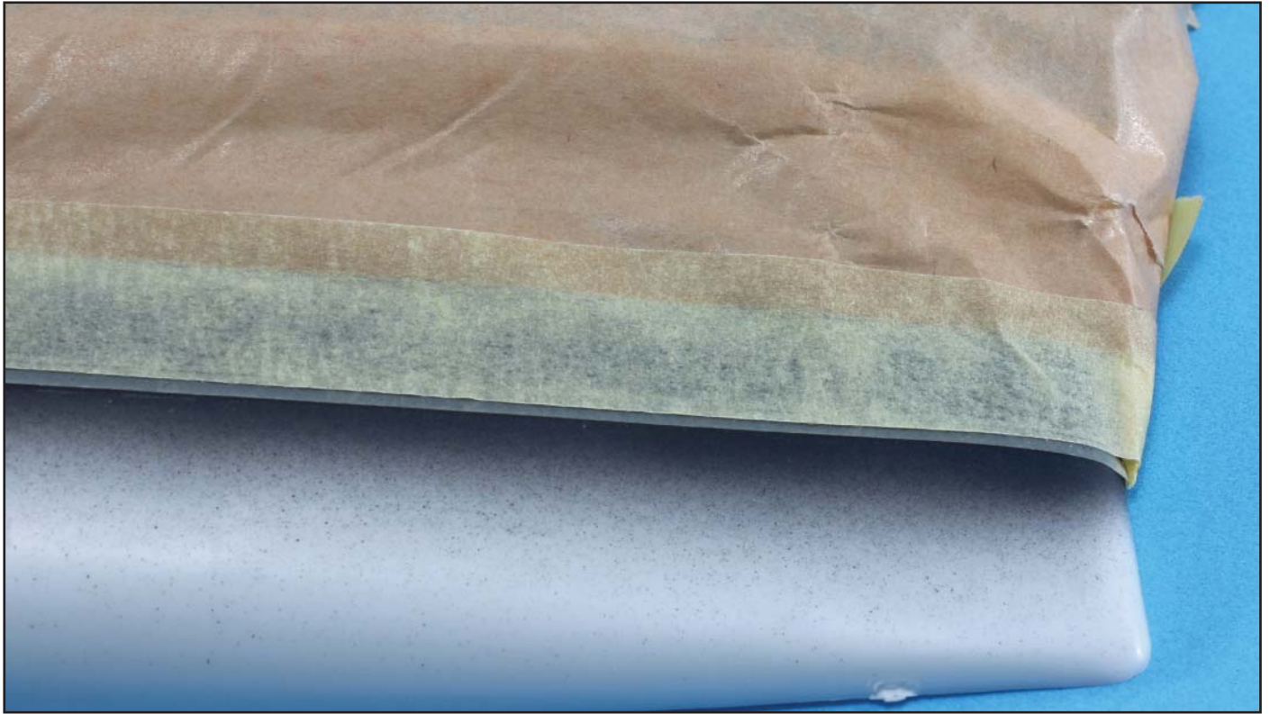
7. Mask off the upper hull using ProMask or tape and paper to mask the upper hull.
