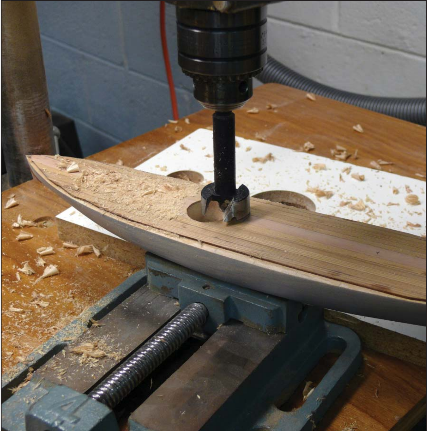
21. Drilling out the cockpit opening. The hull is held in a drill press vise using that piece of plywood in the centerboard slot.
