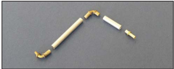
4. Parts of a muffler assembly.
