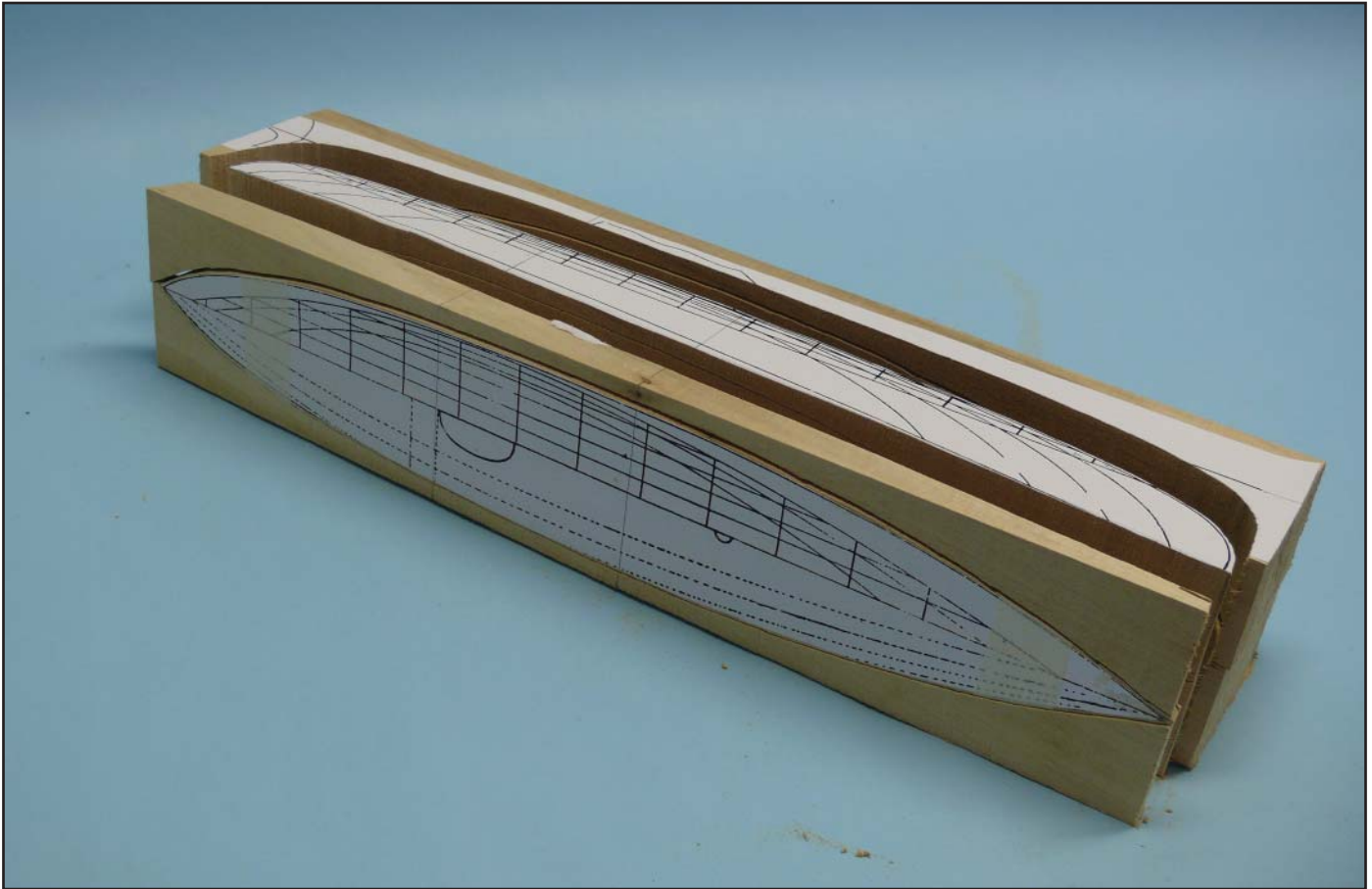
9. Here both the top and profile views have been sawed out and the offcuts have been stacked back together.
