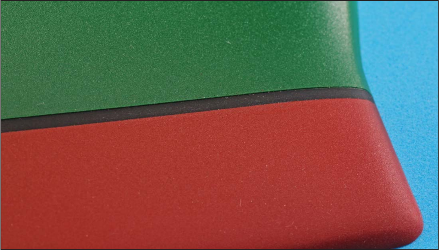
13. Finished paint job after removing the waterline masking tape. Note there is no need for touch up.
