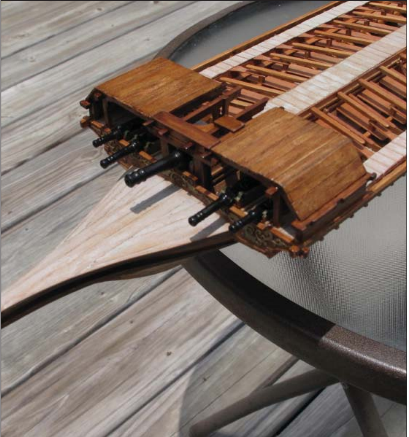
13. Finished forward gun area and foredeck.
