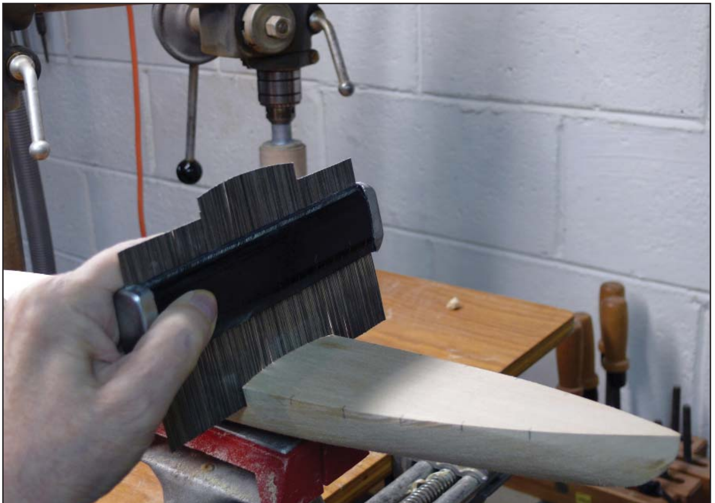
18. Using a contour gage to check symmetry of the deck crown.
