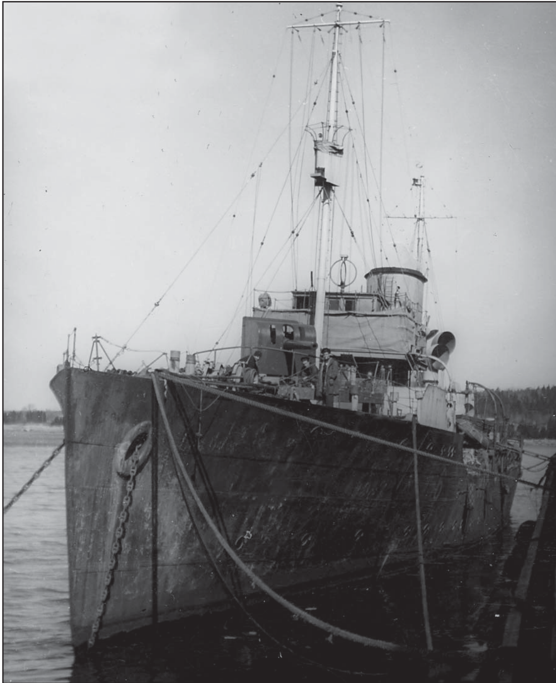
Figure 1 (1941): Chicoutimi shortly after commissioning, at Sydney, Nova Scotia, appears untidy and is painted builder's grey overall. It has the mainmast, and minesweeping equipment will be on the quarterdeck. There may not be any secondary armament. The inadequate size of the original bridge is apparent. All photographs are from the collection of the Naval Museum of Alberta in Calgary, Alberta, used with permission.
