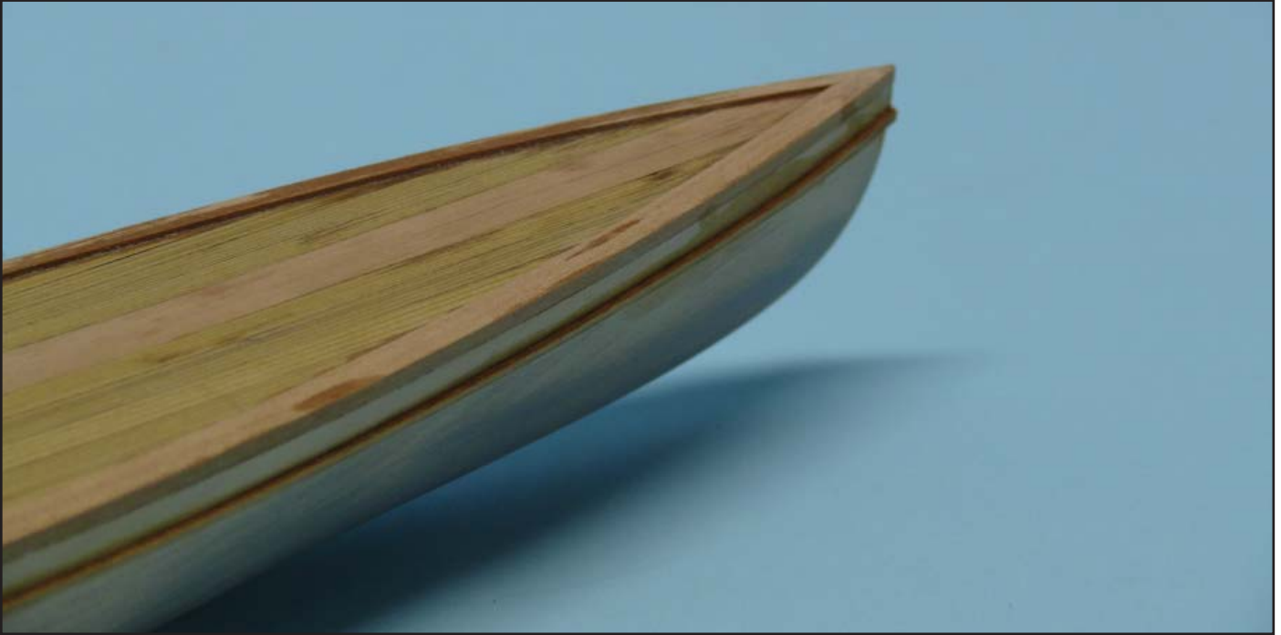
24. Covering boards bonded in place. Note that rub rails, at the level of the sheer plank shown on Martin's plan, are also in place here.
