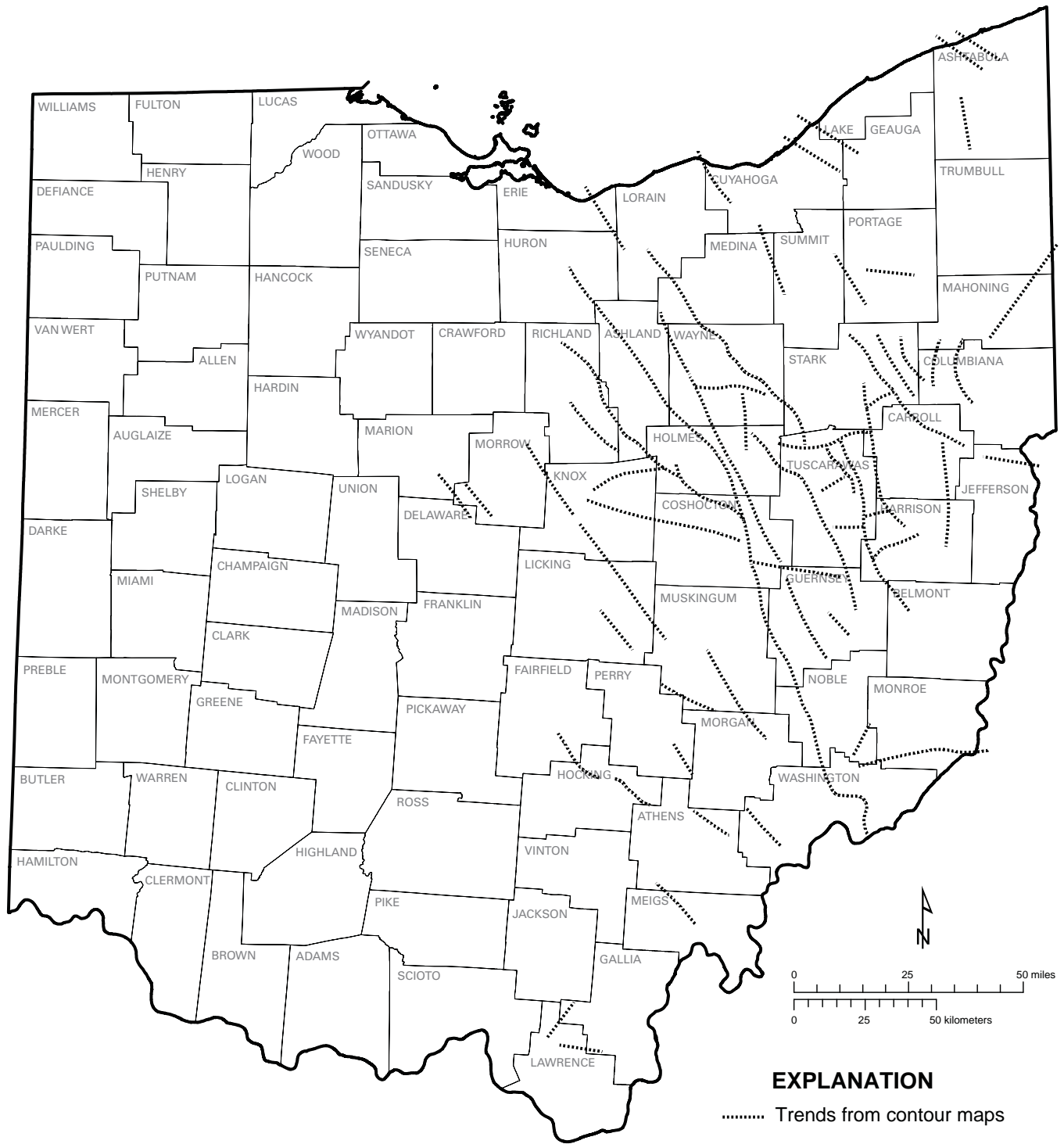
FIGURE 57.—Line map of all trends evident on the surfaces of the Dayton Formation, Onondaga Limestone, and Berea Sandstone; coincident lineaments on multiple surfaces imply a structural plane.
