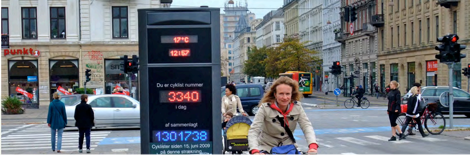
Bicycle counters like these in Copenhagen are increasingly being used in the US to measure bicycle demand on major travel corridors. Image from James Scridland
