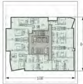
Typical IBC Tower Core Alto - Seattle 8,000 SF Floorplate 12 units per floor 672 ave. unit (gross) 551 SF ave. unit (net) 1387 SF Core = 17%
