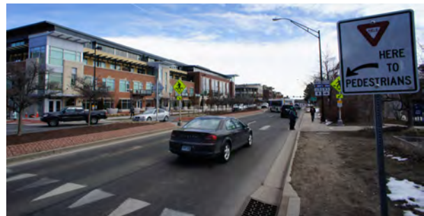
Mid-block pedestrian crossing with rapid flashing beacon in Boulder, CO. Image from Nelson\Nygaard
