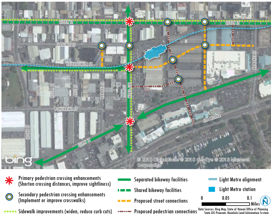
Figure 5-25 Kaka`ako Station Access and Circulation
