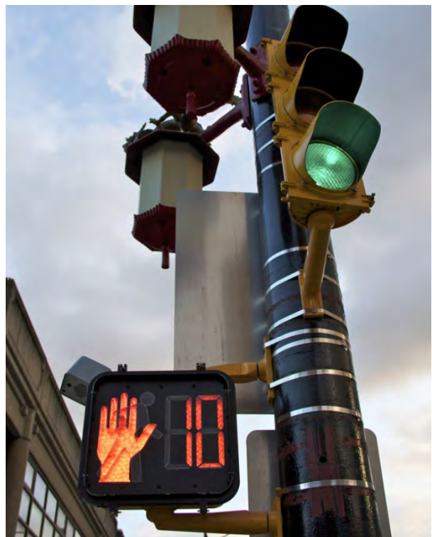
Pedestrian countdown signals can assist help make crossing safer. Image from Nelson\Nygaard
