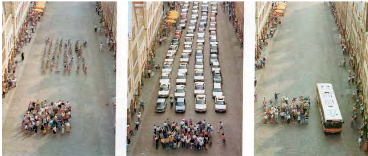
Automobiles require much greater capacity to move the same amount of people than buses, bicyclists, and pedestrians. Image from City of Muenster, Germany
