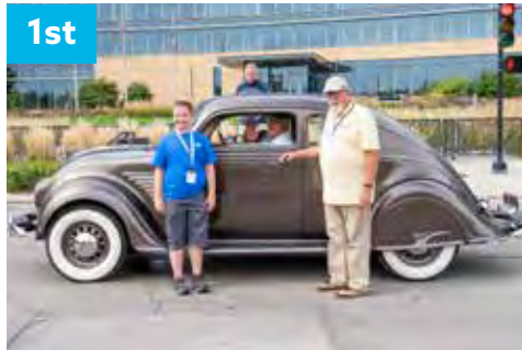
1st 1934 DeSoto Airflow Coupe owned by Fred & Renee Mehr of Cold Spring, MN The Airflow concept was initiated by Chrysler engineer Carl Breer, along with the consultation of Orville Wright. It was the first aerodynamically tested and designed car, and the first car where the engine was over the front axle (allowing passengers to ride between the axles). Only about 15 of these coupes survive.
