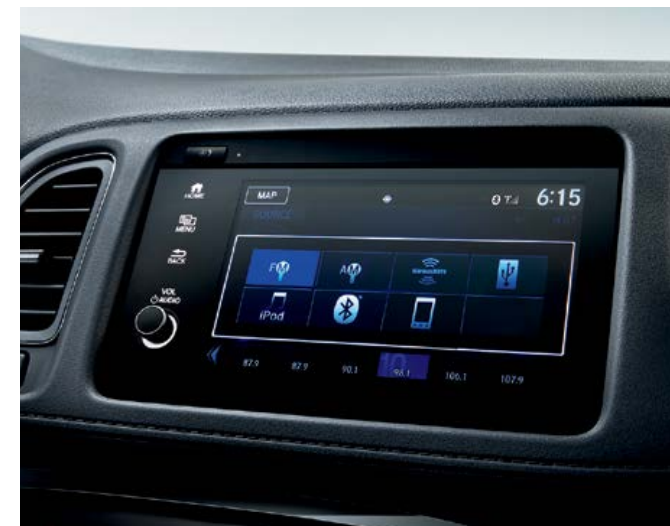
Available 180-watt AM/FM audio system with MP3/Windows Media® Audio playback capability and 6 speakers
