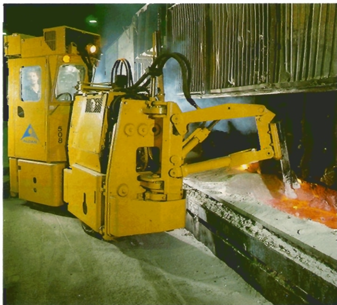
New machines, equipped with air-filtered cabs, are being introduced in Alcan's Quebec smelters as an additional protection for employee health.
