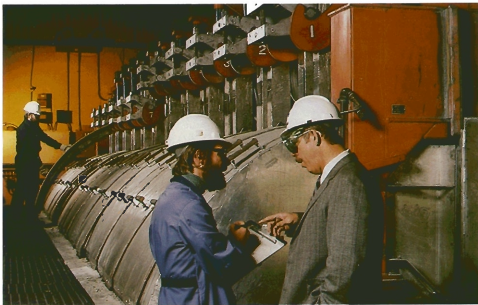
A final prototype of Alcan's newly developed 275-kiloampere electrolytic cell was built and tested during 1984, at the Company's R & D facility in Jonquière, Québec.
