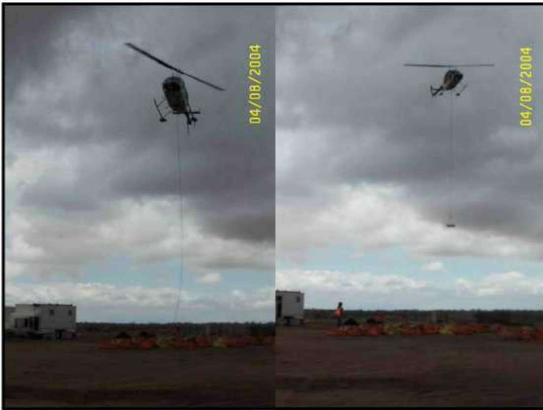
Figure 3-8. Helicopter moving equipment into sensitive areas to avoid environmental harm.
