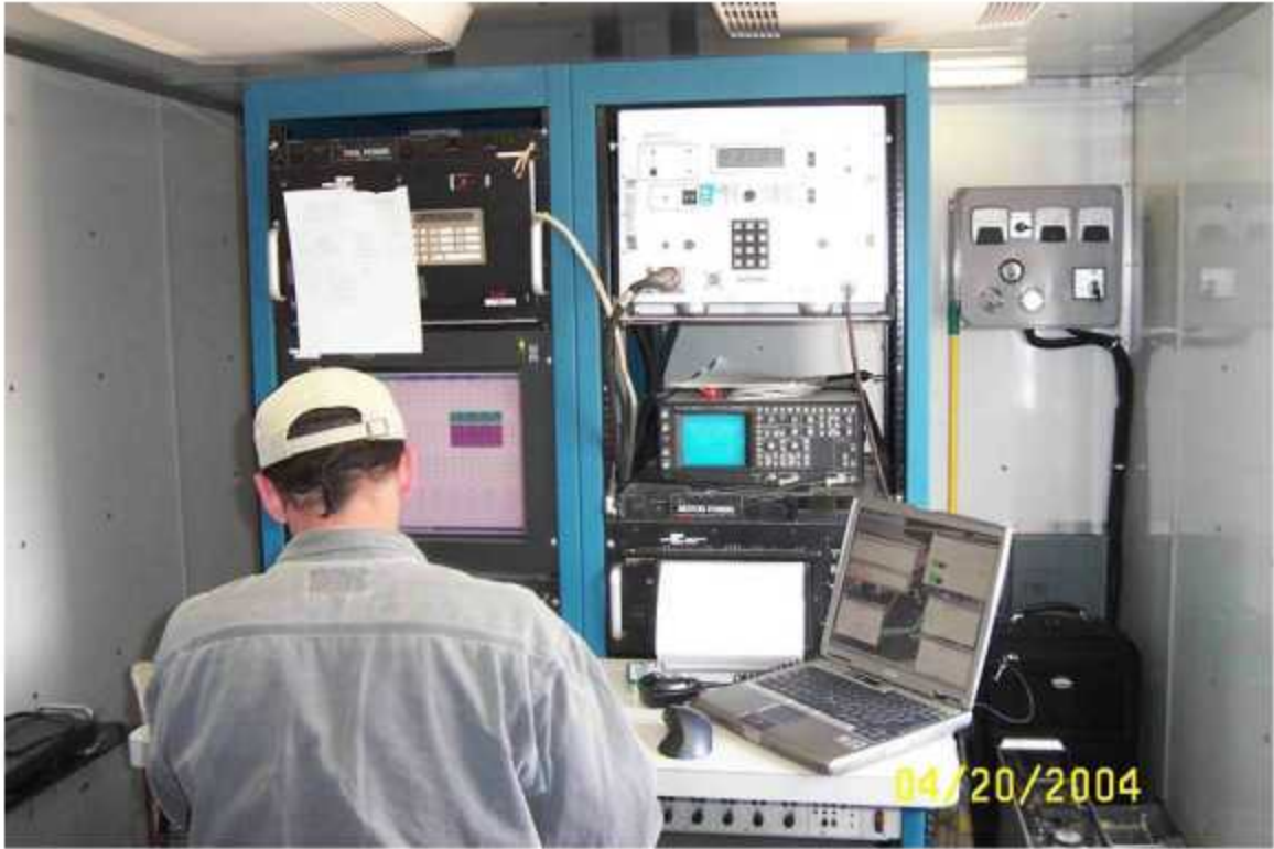
Figure 3-20. Acquiring the VSP data.
