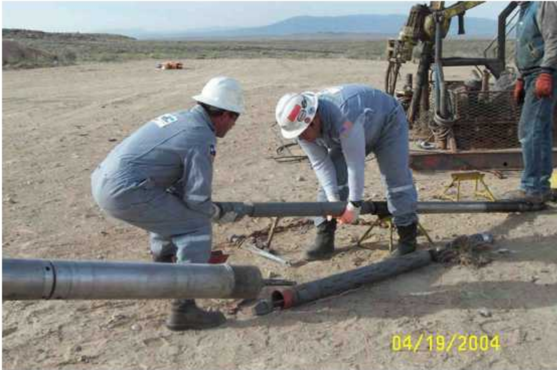
Figure 3-18. Assembling equipment for the VSP.
