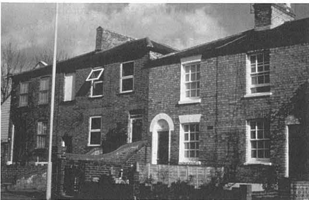
A typical conservation area whose appearance and character is marred by the replacement windows on the left. All photographs by courtesy of English Heritage.
